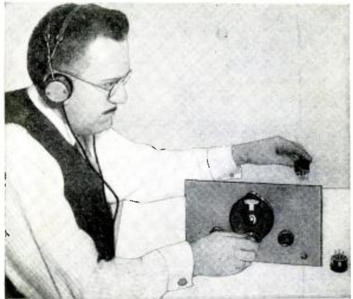
Appearance of Mr. Simmons' 2-Tube Short-Wave Receiver—ideal for the beginner. The cost of the parts is low and the capabilities of the set practically unlimited.
