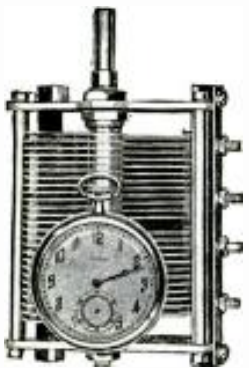
Actual photograph showing relative sizes of watch and Midway condenser. The condenser is a Midway Featherweight 2 gang condenser for broadcast receivers, 375 mmfd. per section 3 3/4" long (back of panel) 3" wide and 2 1/4" high (with plates extended), weight 8 oz. Note sturdy construction.
