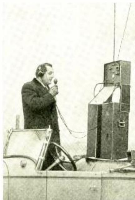
Charles Srebroff, president of the Radio Engineering Laboratories, demonstrating the portable ground station at Curtiss-Wright Airport, North Beach, L. I. Note the di-pole antenna behind the upright case.
