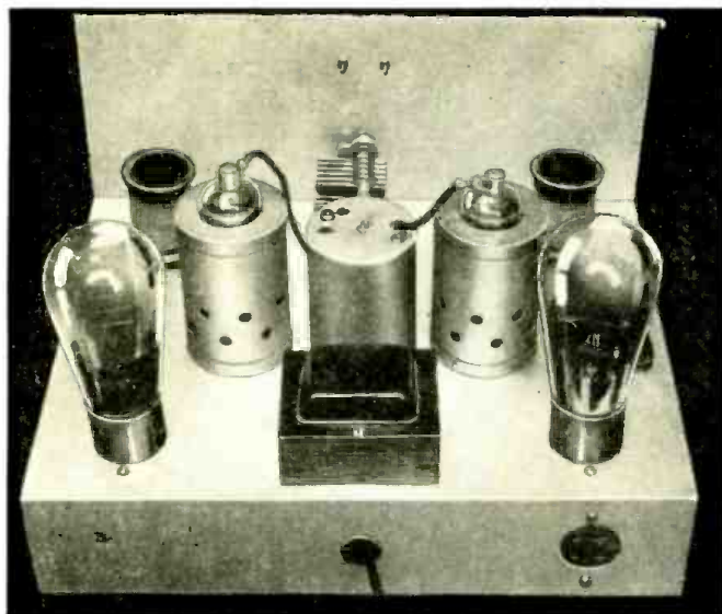
Rear view of the 4-tube Superhet developed by Mr. Denton especially for Short Wave Craft readers; the four tubes include the rectifier. The first detector also serves as the oscillator, operating on the autodyne principle.
