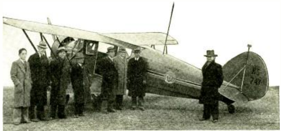
The radio-equipped patrol plane used by the Conservation Department of the State of New York. Note the mast aerial sticking out of the body.
