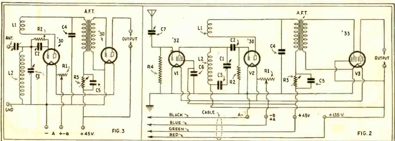
Diagram at left shows the original 2-tube "Go-Getter" hook-up, as given in the March number. Diagram at the right shows the improved modified "Go-Getter" hook-up, incorporating an untuned R.F. stage and a pentode output stage.
