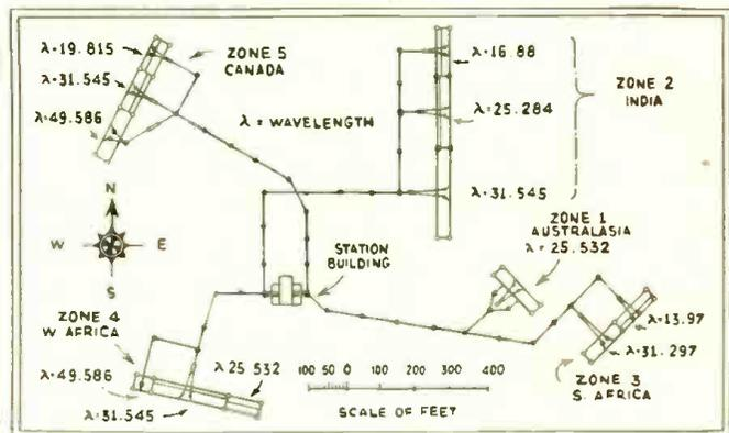
Above—ground plan of the directional antenna arrangements at Daventry, where the powerful short wave beams are hurled to distant climes.
