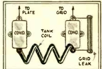
When building a Hartley transmitter, I broke the two insulators used to support the tank coil. Instead I screwed two bakelite fixed condensers to the baseboard and screwed the tank coil onto the ends. As these condensers were necessary as grid and plate blocking condensers I saved space and the cost of two new insulators.—L. Emmett Rhoden.
