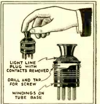
protects the windings from being loosened or pulled off. It does away with the necessity of doping coils; a practice which has been denounced by many successful set designers. Since these outlet plugs can be purchased in four or five colors, the different coils of a set can be distinguished quickly.
