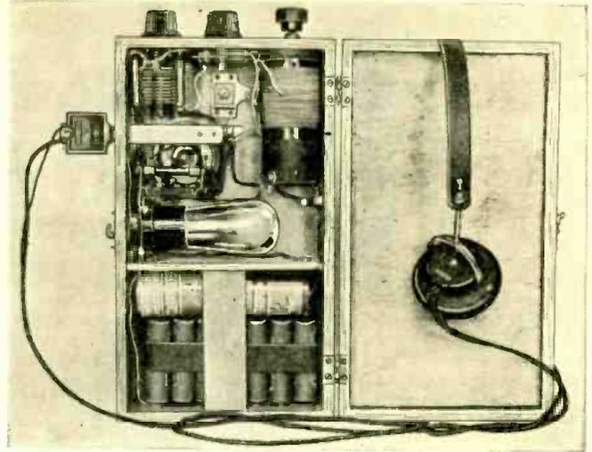
This pocket size receiver employs a standard short-wave circuit with several innovations made by the author. He has arranged the regeneration control in the form of a movable tickler coil; the different wave-bands are switched into or out of circuit by means of a home-made switch. A filament-control jack is advantageously employed.
