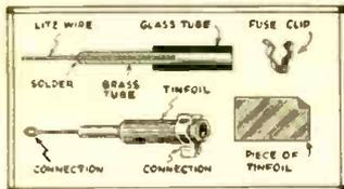
of the connections from the screw that fastens fuse-clip to the base-board. Now, solder a piece of Litz (stranded) wire to a piece of brass tubing that just fits inside of the glass tube; next secure one
