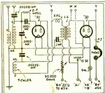
Simple connections used in Mr. Cullen's Short-Wave Receiver, which can be used for most every purpose met with by amateur radio operators.
