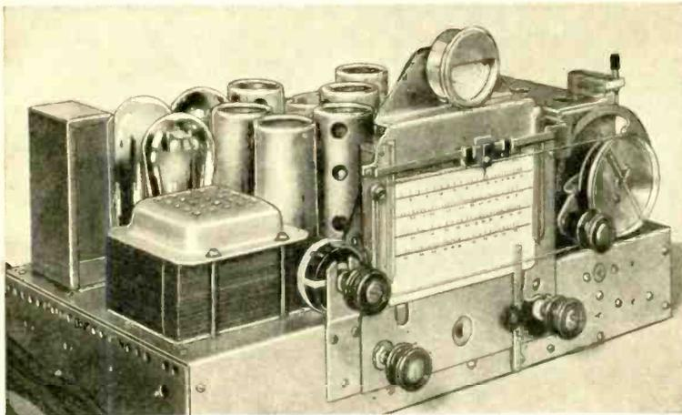
"Close-up" of the 10-tube multi-wave superhet chassis.
