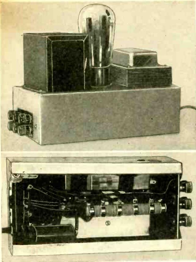
● EVERY short wave experimenter needs a good cheap power supply of small size. I have designed one which can be easily constructed for less than five dollars. It will give 250 volts of pure D.C. at a current drain of 50 milliamperes (more current at a lower voltage) as well as 2.5 volts A.C. at 5.0 amperes. The overall dimensions are only 8½ x 5¼ x 5¼ inches (without the tube).
