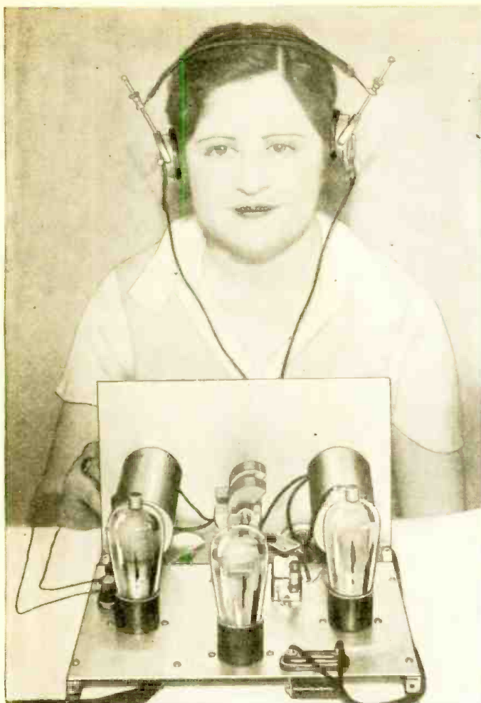
Here's a 3-tube short-wave receiver that you will derive a lot of pleasure from—it is up to the minute, with all controls mounted on the front panel, while switches change the wave bands.
