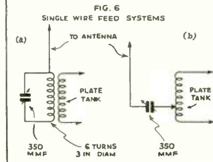
The diagrams above show the Zepp antenna; single wire feed; antenna-counterpoise system, current feed coupling method, and different forms of voltage feed coupling.
