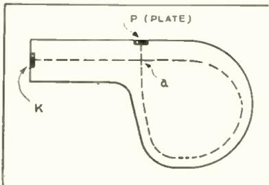
Here is a "Grid-less" ultra short-wave transmitter tube, in which the electronic current reacts upon itself, as shown by the circular dotted line.
