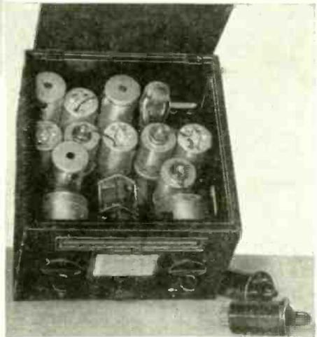
Photo directly above shows the National SW-3 type receiver, four of which are assigned for use on Byrd's planes.
