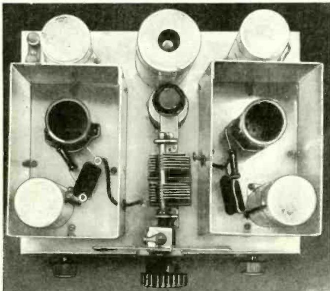
Left — Looking down on Mr. Malsberger's 5-tube SW receiver. The shielding of the various tubes and coils has been carefully worked out by the designer, and particular care and research given to the form of circuit used.
