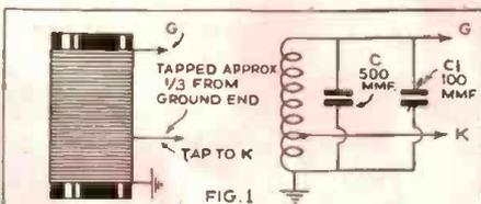
BEAT OSCILLATOR COIL MADE FROM SECONDARY WINDING OF AN R.F. COIL, SHUNT WITH A .0005-MF. MICA CONDENSER AND A .0001-MF. PADDING CONDENSER.
