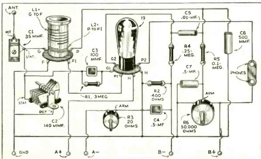
Pluri-tized wiring diagram which even the most inexperienced short-wave fan can follow. In order to build this excellent one-tube receiver which gives 2-tube results.
