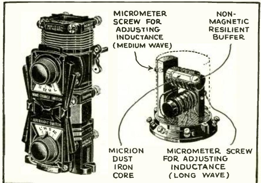
The latest European design of short-wave tuning couplers are shown above; apparatus at right (A) has coils fitted with special "iron dust" cores, designed for use at high frequencies; (B) left, shows "All-Wave" coupler.
