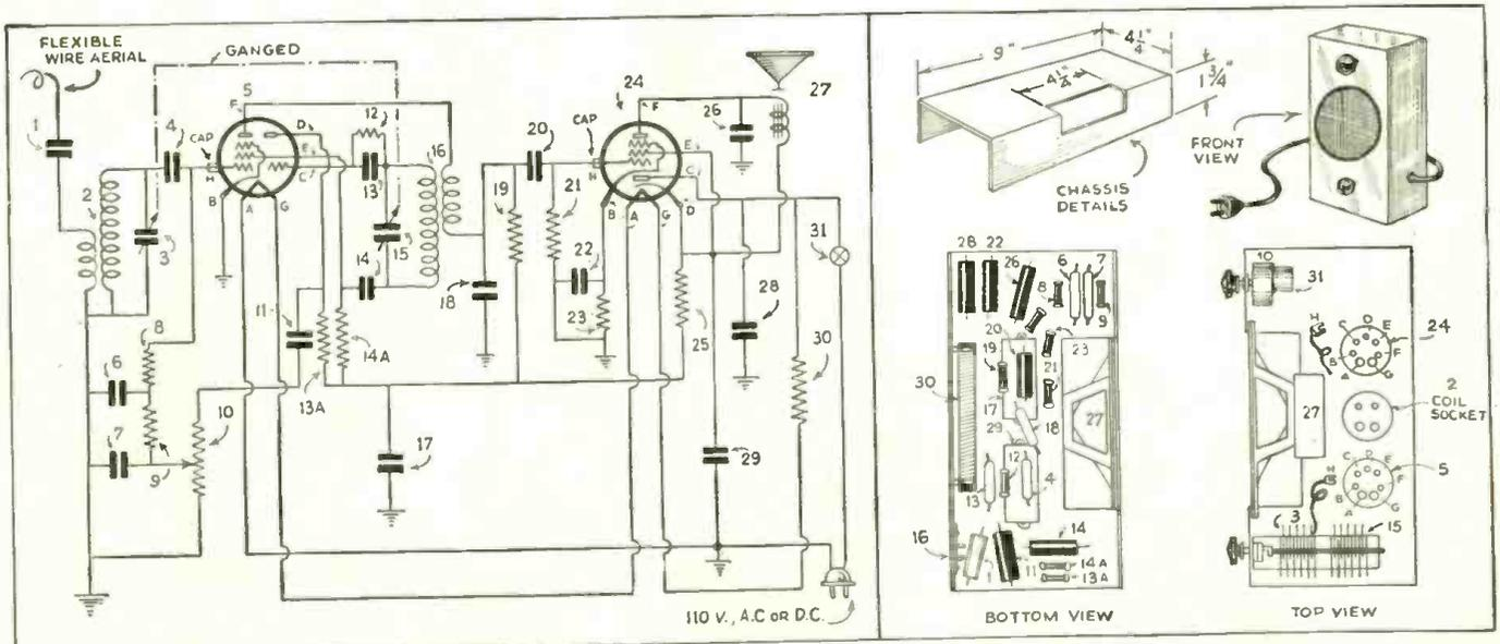
Constructional details including wiring diagram for building the 1934 2-Tube "Pal" Portable—a pocket-sized set designed to operate on 110 volt A.C. or D.C. circuits.
