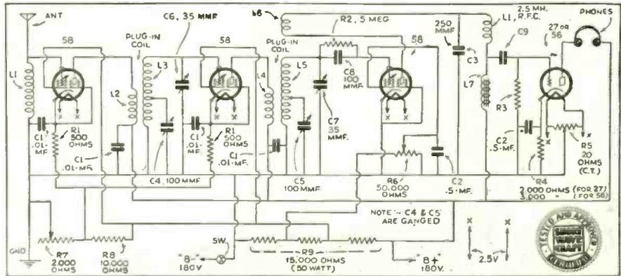
Schematic wiring diagram for the 4-tube receiver employing two stages of R.F.
