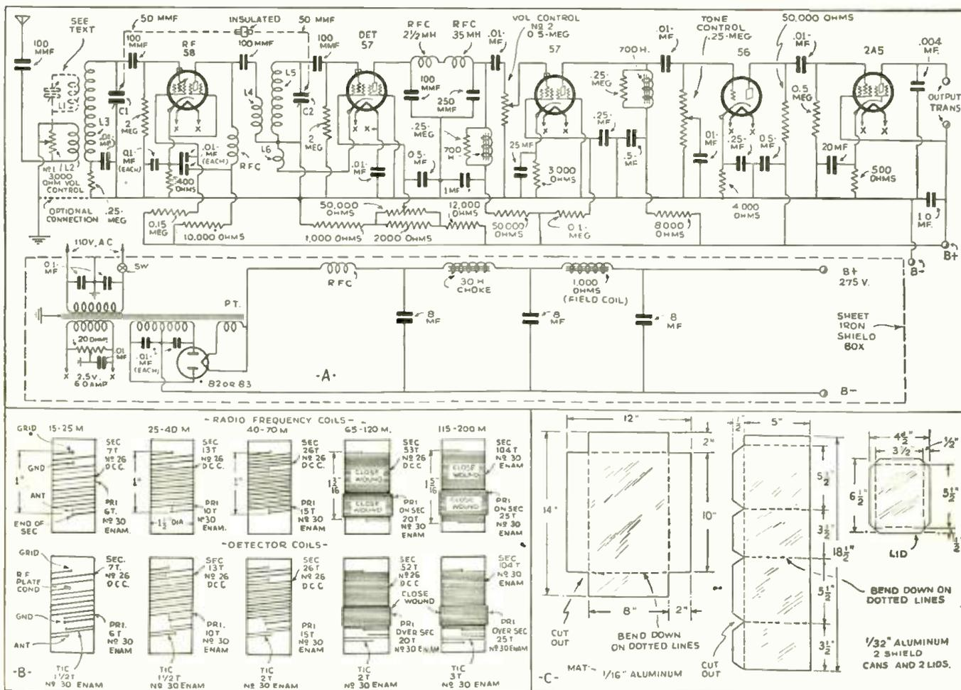
Coil data and scheme of connections for the "Advanced" 5-Tube Receiver.
