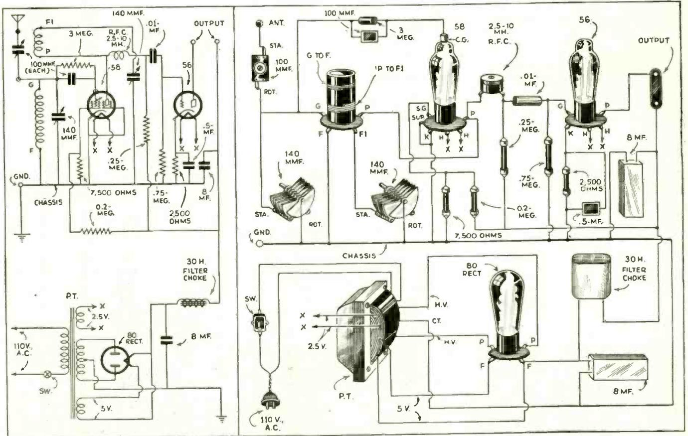
Complete schematic and picture wiring diagram, enabling anyone to build the 3-Tube Short-Wave Receiver here described. It operates on your 110 volt A.C. lighting system—no batteries required and it will haul in the "foreign" stations like nobody's business.
