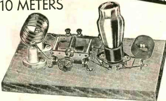
Paradoxical as it may sound, this ten meter transmitter EMPLOYS A SINGLE TUBE IN PUSH-PULL ARRANGEMENT. Heretofore the word "push-pull" automatically implied the use of two tubes, yet here we are with a one tube push-pull transmitter.
