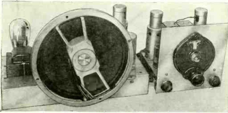
General appearance of the beat oscillator, audio amplifier, and power supply unit, at left; original "2-Tube Superhet" unit at the right.
