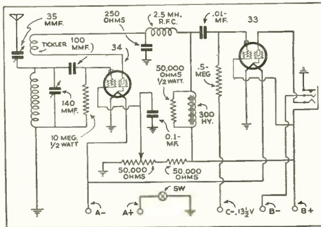
Wiring diagram of "Pretzel-Bender Two".
