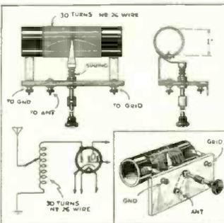
each coil. It should be mounted away from the panel. Use a 1/4" dowel for a shaft. A snug fit on the coupling saves bother with set screws. The center bearing and shaft was taken off an old three-circuit tuner; the contact arm from a rheostat. Between 30 and 35 turns of about No. 26 enamel wire used.—Ralph S. Thompson.
