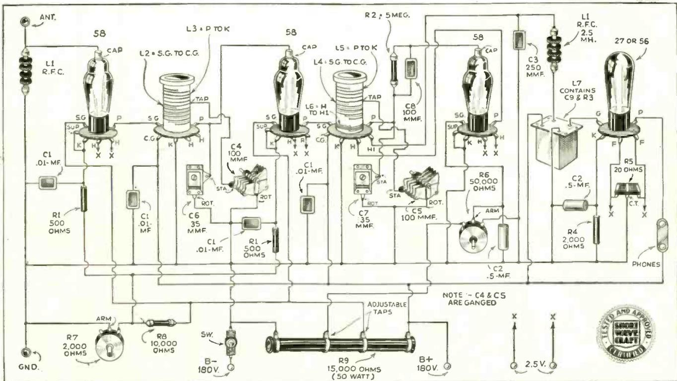
It's a "clench" to build this dandy 4-Tube Receiver. with its exceptionally high sensitivity for weak or distant signals, by following the picture diagram presented above. The tuning of the set is simple and it will undoubtedly make many friends.
