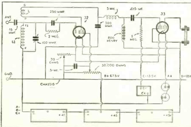
Schematic wiring diagram for the Fultone II—a 2-tuber.
