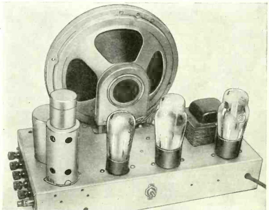
Top view of the beat oscillator, audio amplifier and power supply unit.
