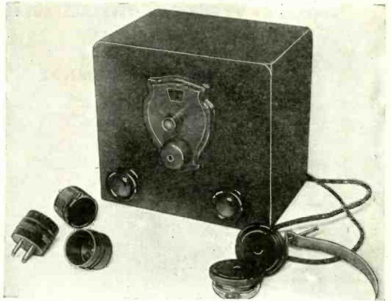
This battery operated short-wave receiver employs plug-in coils and uses but two "low-drain" 2-volt battery tubes to give a good "healthy" signal in the phones.
