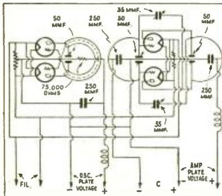
Physical appearance and wiring diagram of 5 meter transmitter (No. 145).\*
