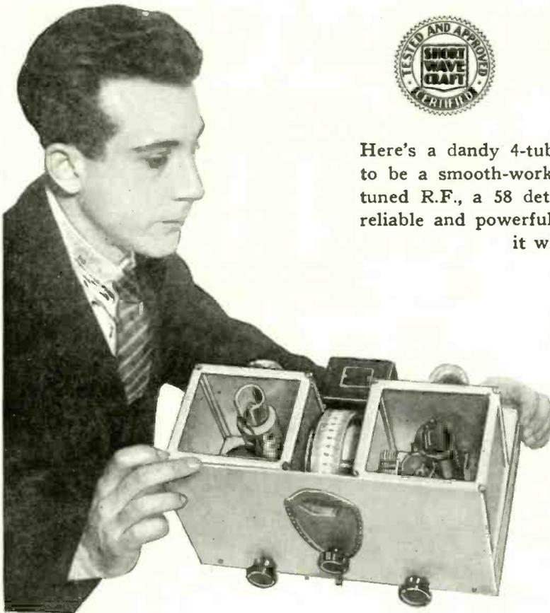
Here's a dandy 4-tube receiver which tests have repeatedly shown to be a smooth-working job. It employs a 58 untuned R.F., a 58 tuned R.F., a 58 detector and a 27 audio stage. It makes a very reliable and powerful headphone receiver and under fair conditions it will work a loud speaker nicely.
