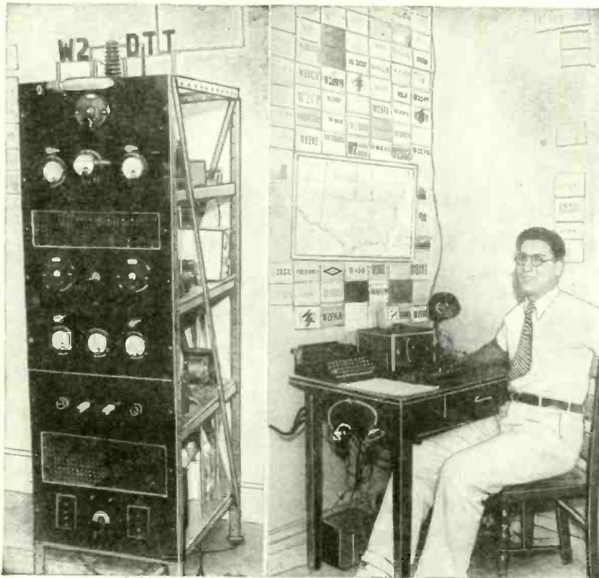
The complete 250 watt crystal-controlled transmitter owned and operated by Alvin Abrams in New York City under the licensed call of W2DTT. Mr. Abrams is observed seated at his operating desk, together with a small part of the great number of QSL cards he has received from all parts of the world.
