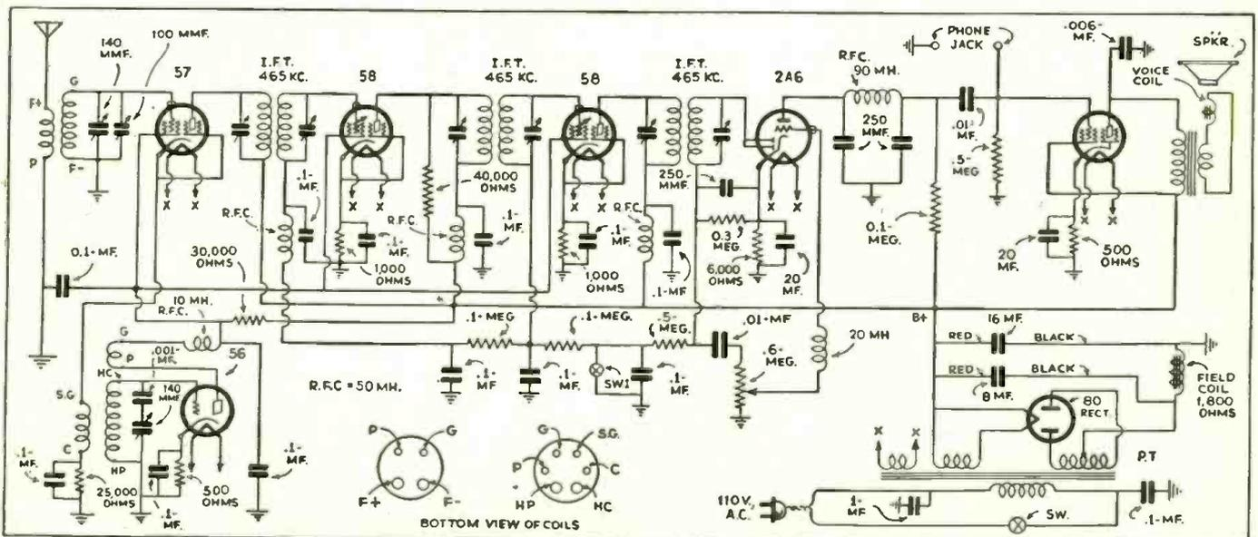
Schematic diagram of the Superba Short-Wave Superheterodyne.
