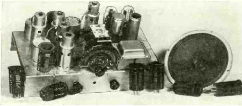
This photograph clearly shows the neat arrangement of parts used in this modern short-wave superhet.
