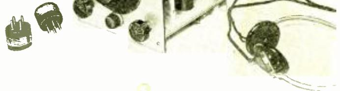
The 2-Tube "Easy-Tune" Band-Spreader here illustrated is intended primarily for headphone reception and makes a dandy job for those just starting in the short-wave game. A rear view of the receiver is shown at left.
