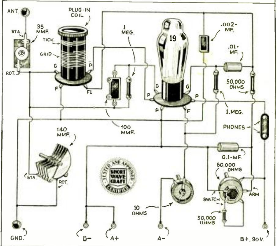
Practically anyone can follow the extremely simple wiring diagrams given above, both in schematic and picture style, so that they can enjoy the really surprising performance afforded by this ideal 1-tube set, which employs a single 19-tube. The set works on a 2 volt "A" battery.
