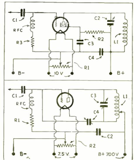
Those interested in Mr. Alvin Abram's article on a 250-watt transmitter, page 661, March issue, will most probably have noted that the center tap connection to the filament resistors, R1 and R2, figures 3 and 4, were not completed. They are shown correctly in the diagrams herewith.
