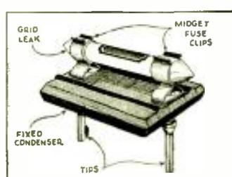
**PLUG-IN "GRID-LEAK AND CONDENSER"**
