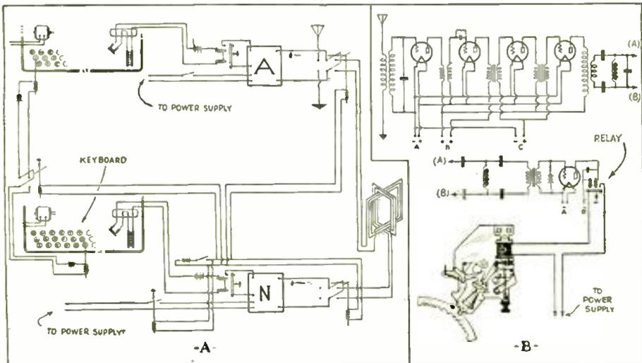
Above—Diagram of general arrangement of the Sibley teletype system; at right of diagram, typical radio receiving circuit for teletype signals is illustrated.
