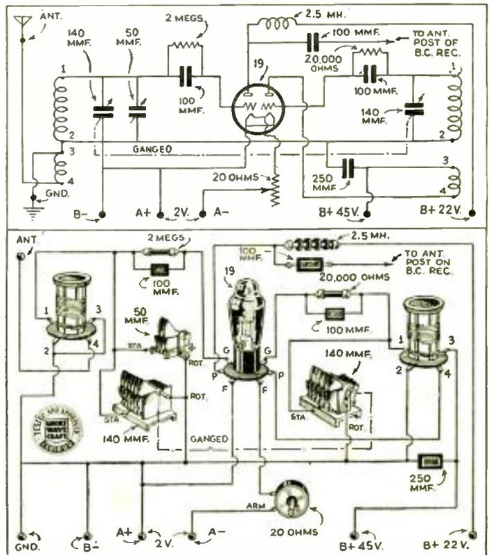
Both schematic and picture diagrams have been laid out by the author as shown above, so that even the tyro can build it.
