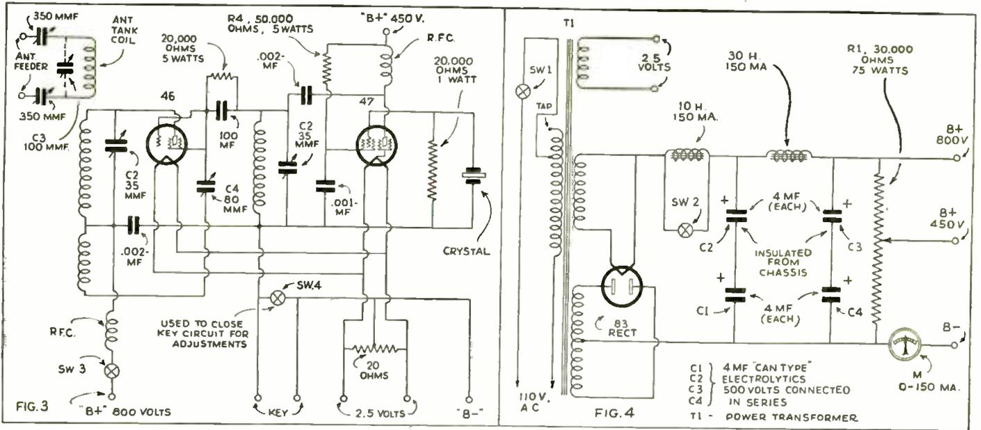
Wiring diagrams of crystal controlled M.O.P.A. and power supply.
