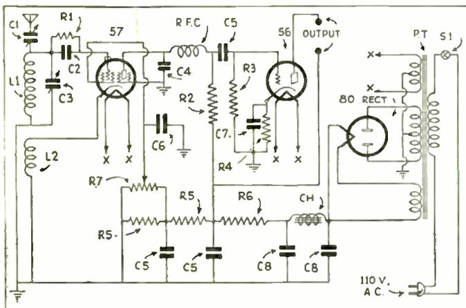
Wiring diagram used in assembling the "International 3".
