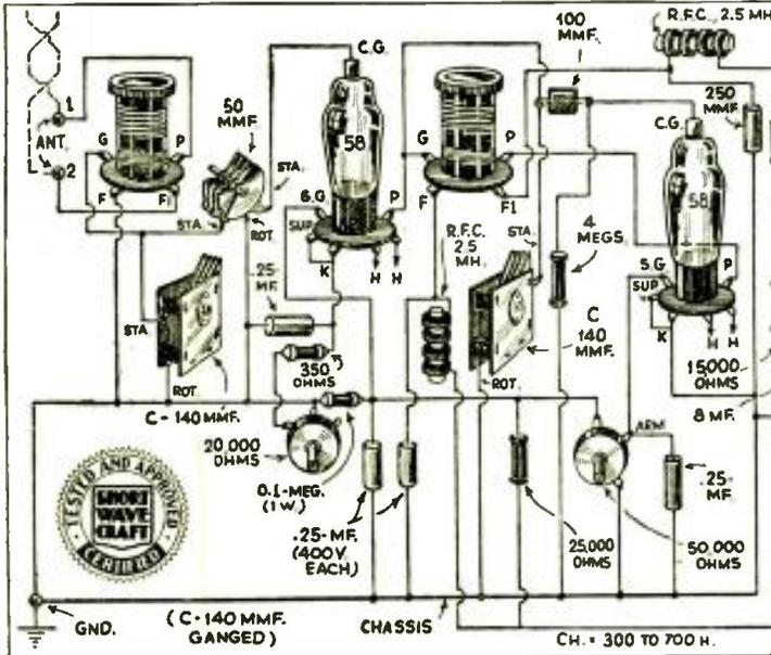
Above: Schematic wiring diagram of the "RGH-4" All-Wave Receiver here described by Mr. Herzog. The tubes and the circuit worked out by Mr. Herzog result in a very strong signal at the loud speaker. Of course, a sensitive, small-sized speaker is to be preferred for use with any set of this type. Left: Picture wiring diagram of the "RGH-4"—it uses but four tubes, one of which is the rectifier. The "RGH-4" can be built at a reasonable cost.
