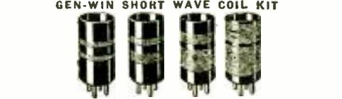
These coils are considered the finest made. Each coil is Precision wound on a different colored baseplate form for quick identification of wave lengths. Used and highly recommended by all short wave experts. Range (16 to 225) meters, using a .00014 or .00015 mfd. condenser. Recommended for the following sets: "The Duke Trotter," "The Osceola," "The Iberia 12,500 Mile Two Tube Receiver and Iberia Three Tube Signal Gripper," "The Mesadyne."
