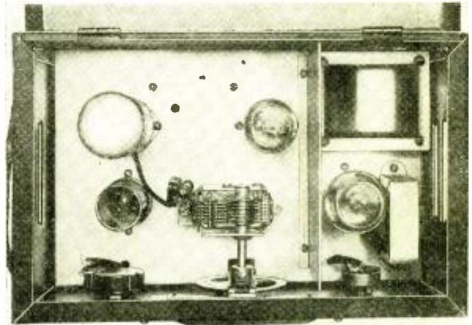
Top view showing tubes, coil, and tuning condenser.
