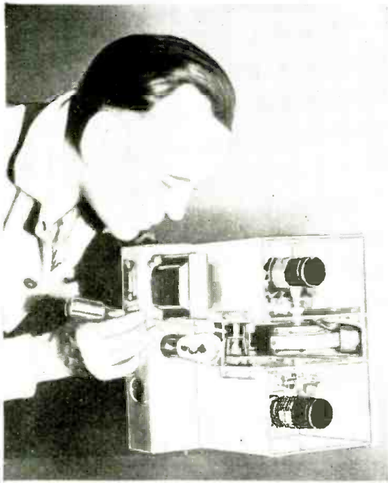
Fig. 7. No shielding is necessary for the portion of the R.F. tube between the cabinet knobs compartments. Right: Panel view of receiver; while 5 knobs appear the instrument has single dial control. Fig. 1.
