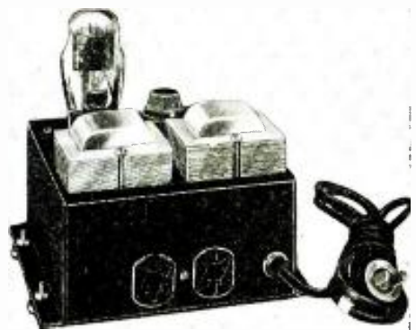
The Phantom Cell—the approach of a body causes a bell to ring, etc. No. 318.
