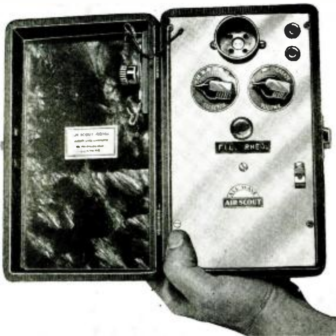
Isn't this 1-tube receiver a dandy! And the "A" and "B" batteries are all self-contained in the small cabinet, which can be held in one hand, as the photo shows.
