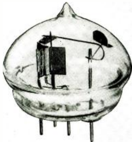
The 316-A triode shown above, will work at frequencies as high as 750 megacycles.
