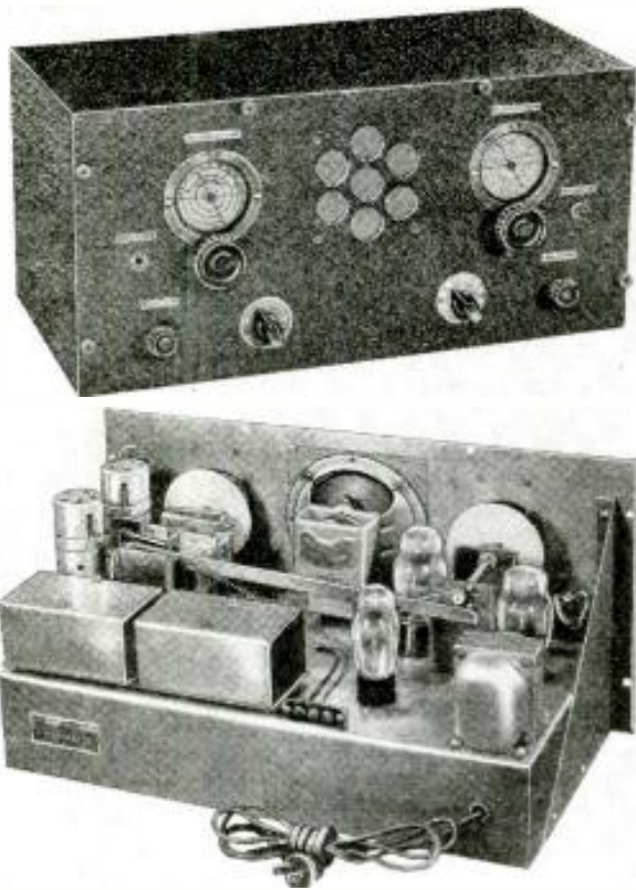
Above—Front and chassis views of the Sargent Model 11 T.R.F. receiver, available in ranges as great as 9.5 to 20,000 meters. (No. 584)
