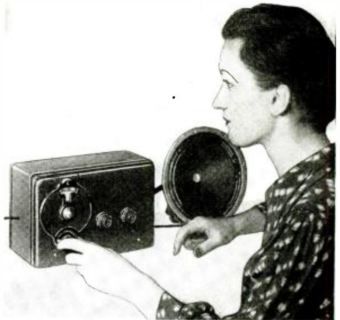
The 5-meter superhet pulling in "Ham" phone stations.
