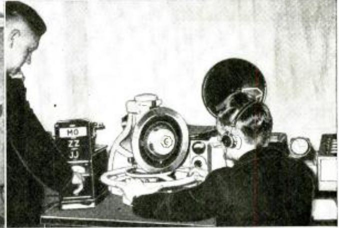
The photo at left shows short-wave transmitter by means of which the operator gives the airplane pilot his exact position. Photo at right shows new German short-wave apparatus used to guide flyers. The wheel shown in the photo rotates the directional antenna on the roof of the building.
