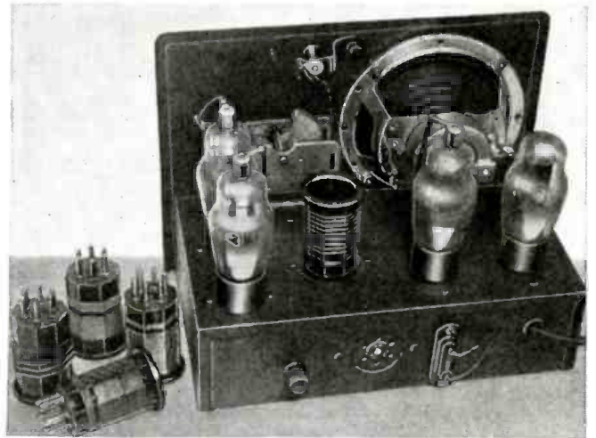
A peek at the rear of the "Universal" set. Plug-in coils cover all bands.
