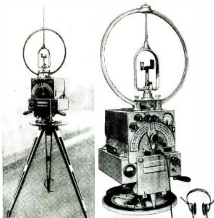
The photos above show the new short-wave surveying instrument used by the German army. It is a thoroughly portable device and has a very high accuracy.
