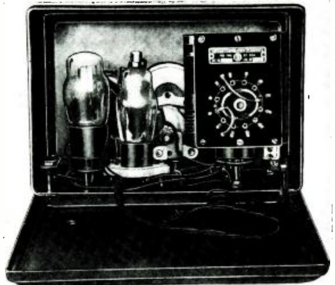
Photo above shows a rear view of the 2-volt receiver, which covers 16 to 550 meters with a handy band-switch.
