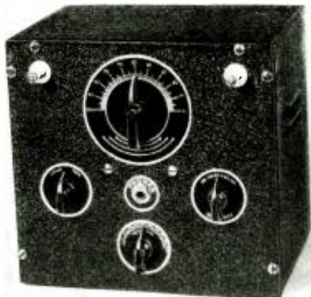
New Trans-Receiver which has a receiving range of 2.5 to 4,000 meters. (No. 623.)
