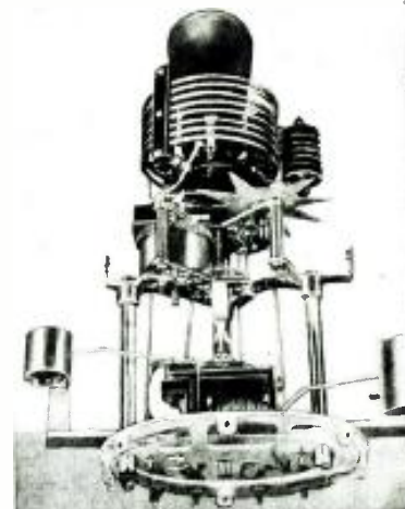
View of another type short-wave transmitter carried aloft by weather balloon.
