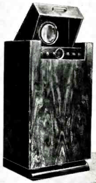
Fig. 4—The Radio L.L. television receiver, with vertical cathode-ray tube.
