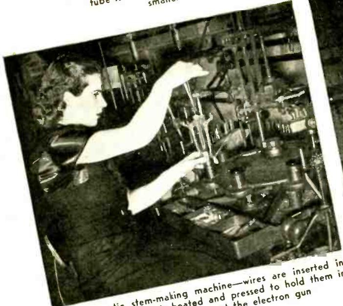
The automatic stem-making machine—wires are inserted in a glass collar, which is heated and pressed to hold them in place. This unit will support the electron gun and deflection plates.
