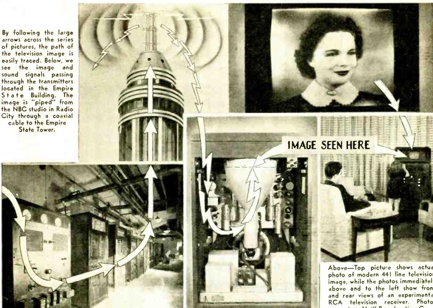
Above—Top picture shows actual photo of modern 441 line television image, while the photos immediately above and to the left show front and rear views of an experimental RCA television receiver. Photos courtesy Nat'l Broadcasting Co.
