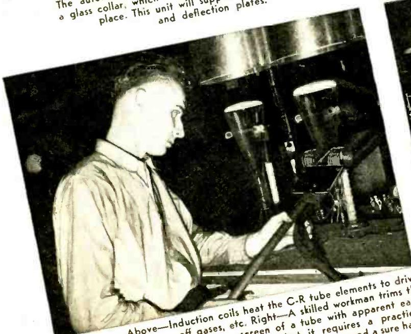
Above—Induction coils heat the C-R tube elements to drive off gases, etc. Right—A skilled workman trims the screen of a tube with apparent ease, but it requires a practiced eye and a sure hand.
