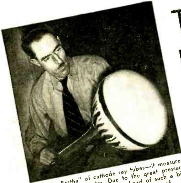
The "Big Bertha" of cathode ray tubes—it measures 13½-inches in diameter. Due to the great pressure exerted by the atmosphere, the head of such a big tube is made rounder than in the case of smaller size tubes.
