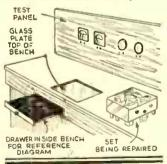
bench is usually littered with tools, solder, etc., and the large service manual would be in the way. Therefore, I have cut a slot in the front of my bench about  $\frac{1}{2}$ " below the top. Instead of a drawer, I put in here two sheets (Continued on page 633)
