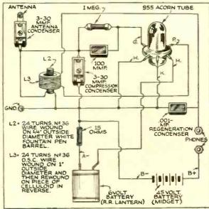
size to slip over the grid coil. Both coils are kept in position with fingernail polish, used as a lacquer. The grid coil is a straight solenoid; the jumble-wound tickler is slipped over and adjusted for best volume.
