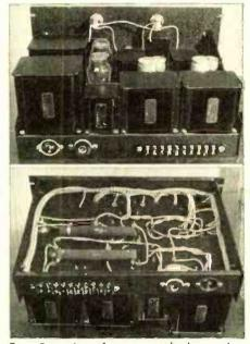
Top-Rear view of power supply. Lower view shows under side of same.
