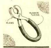
ing around live wires and also when a number of small parts must be picked up in rapid succession, or when the pliers must be opened and closed frequently, as when screwing a nut tight in a cramped space.—David Lloyd.
