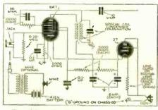
The pick-up is plugged into the jack provided for it and the radio tuned to the low-frequency end of the dial (around 600 kc.) where no station is heard and the turntable is then started. The condenser is varied by turning the adjusting screw until the record is heard through the loud-speaker with the volume control well up.
