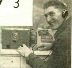
Because of the high amplification factor of the 1A5-G output tube, almost as much volume can be obtained from the single pentode as would be produced by two tubes such as the type 30 or 1H4-G. If a sensitive, high-impedance speaker is used, most of the more powerful stations can be brought in with fairly good volume. However, the receiver, as shown here, is designed for headphones rather than a speaker.
