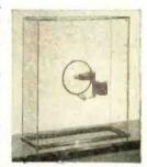
a loss of permeability which, in turn, unbalances the lines of force from the magnet, causing the disc to revolve at the rate of about 20 r.p.m.
