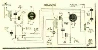
Circuit for 21/2 meter Transceiver. No. 1168.
