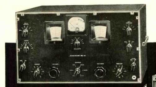
Tuning range: 31-54 megacycles (9.7-555 meters). Complete with crystal, tubes, and 10" "PM" dynamic speaker at a price well within reach of the Ham and Fan.
