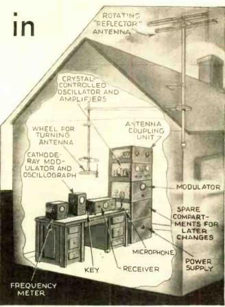
As our cover picture shows, the rotary beam aerial is being widely used by advanced Ham stations.
