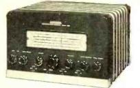
THE accompanying picture shows one of the newest communications receivers—the new Howard model 438. This receiver employs eight tubes and features R.F. amplification on all bands. It uses ceramic coil forms and micalex insulated tuning condensers. Other features include electric band-spread and a crystal filter. The frequency coverage is complete from 540 kc. to 43 mc. in four bands.
