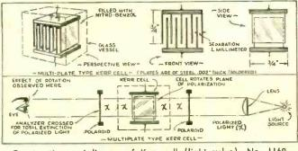
Construction and line-up of Kerr cell (light valve). No. 1169.
