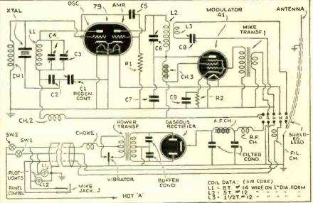
voltage only when desired. Voice currents are fed via the same cable to the modulator. Lights indicate the condition of the switchoperated circuits.
