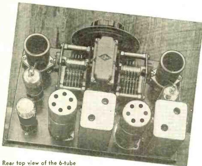
Rear top view of the 6-tube receiver.
