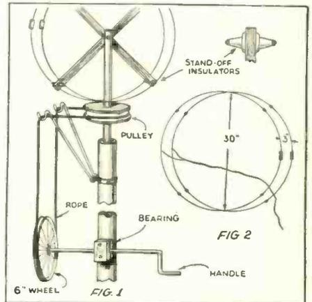
Fig. 1. The construction of the 56 Mc. Rotating Beam.
