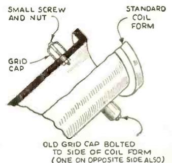
the coil. All that is necessary when changing coils is to pull the feeders, which are terminated in insulated grip cap connectors, yank the coils and substitute the new ones. —Richard L. Kile, K6QPG.
