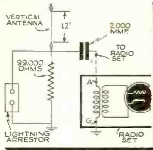
Diagram for Vertical antenna, No. 1174.
