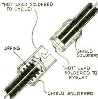
for microphone or phonograph pick-up, can be easily and quickly made with male and female parts of an auto antenna connector. The wires are soldered to the insulated plugs. The shield is soldered to the case of the units.
