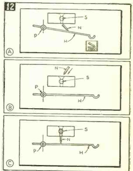
You will notice the handle, pivoted at B, returns to position so that, as shown in Fig. 12C, it forms a gauge permitting the needle to extend the correct distance and no further.
