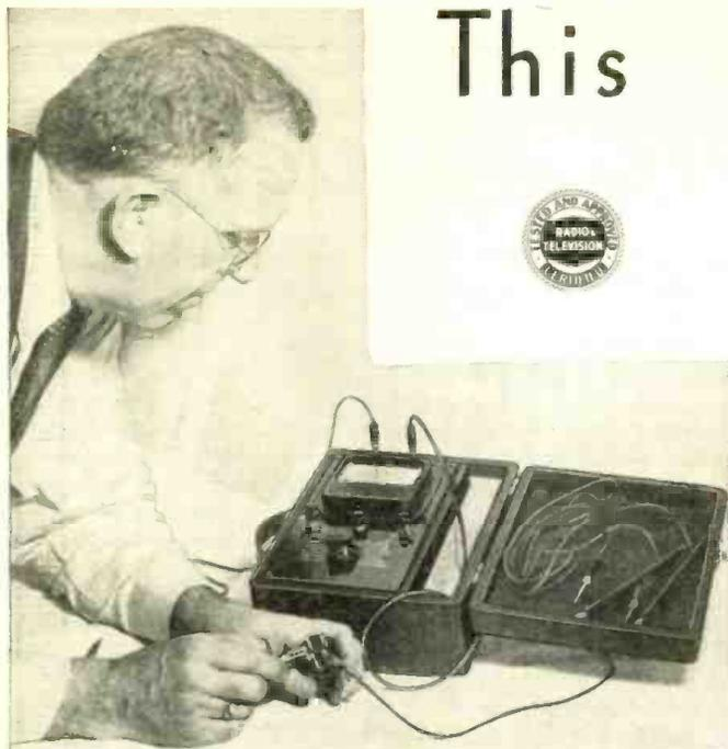
This test meter can be built at nominal cost. It has A.C. and D.C. ranges of 0-10, 50, 250, 1000 and 2500 volts. Current ranges are 1, 10, 50, 250 ma. Three resistance ranges are incorporated. Special scale to fit standard meter accompanies this article.
