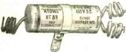
450 V. 8-8 mf.; a 50 V. 10-10 mf.; 200 V. 16-16 and 8-16 mf. units; a 250 V. 6-18 mf.; and 450 V. 8-16 mf. The condensers are hermetically sealed.
