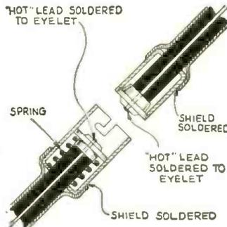
for microphone or phonograph pick-up, can be easily and quickly made with male and female parts of an auto antenna connector. The wires are soldered to the insulated plugs. The shield is soldered to the case of the units. —Raymond T. Stephens.
