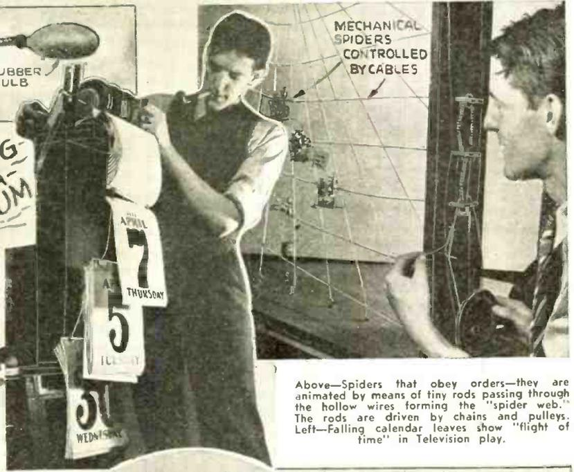
Above—Spiders that obey orders—they are animated by means of tiny rods passing through the hollow wires forming the "spider web." The rods are driven by chains and pulleys. Left—Falling calendar leaves show "flight of time" in Television play.
