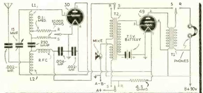
Transceiver for 2.5 meter communication, No. 1176.
