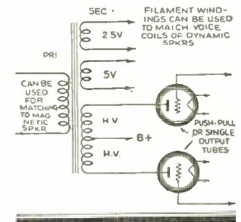
match dynamic speaker voice coils or magnetic speaker windings to push-pull outputs. The various windings are shown in the accompanying sketch.—*H. H. Bloom*.
