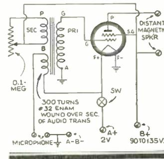
station. The accompanying illustration shows the circuit. The transformer can be purchased, or may be made by winding about 250 to 300 turns of No. 32 enameled copper wire over the secondary of an ordinary audio transformer. The metal chassis is used as a common ground. Plenty of volume and good clear output are secured with 90 to
