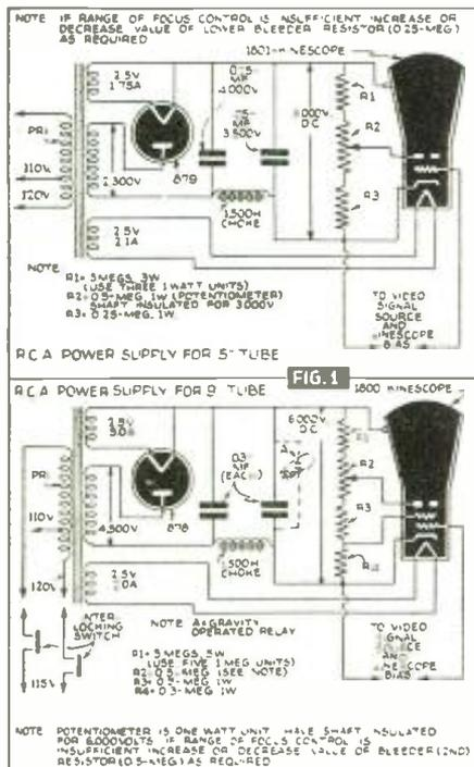
IN the previous chapter of this course we have discussed several types of sweep circuits that can be used in modern television receivers, together with a synchronizing impulse separator. Fig. 1 of this chapter shows two types of power supplies—one for the five inch, the other for the nine inch electro-magnetic deflection tubes.
