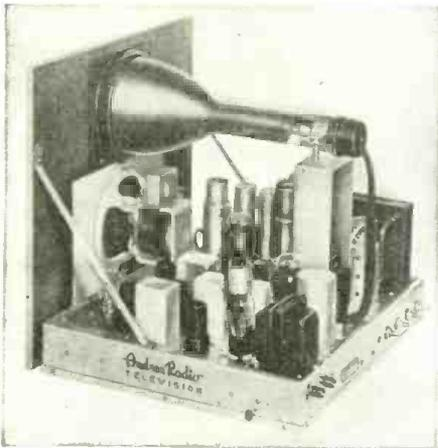
Completed receiver, showing position of tubes, speaker and brackets.
