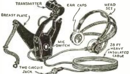
**THIS** Microphone and telephone headset outfit was built especially for the U. S. Navy Aviation Corps.
