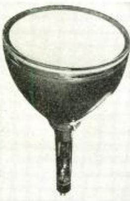
The other accompanying illustration shows the Philco tube with the *flat screen*. The glass end of this tube is approximately  $\frac{1}{8}$  of an inch thick.
