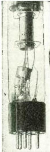
**T**HE ELECTRON GUN in the new Philco cathode-ray tube is shown in close-up at the extreme left. You will notice that the gun is offset so that the ions which normally cause *ionization blemish* on C-R screens pass harmlessly to one side. The electron stream itself is magnetically deflected in the usual way.
