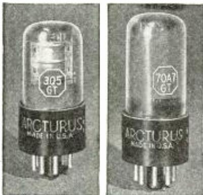
Arcturus' new beam power amplifier, type 3Q5GT, is a filament type beam output unit having a center point connection to filament, which makes possible either a series or parallel arrangement of the two halves. Filament voltage is 2.8 volts for series filament operation and 1.4 volts for parallel filament operation. Filament current is 0.05 ampere for series and 0.10 ampere for parallel filament operation.
