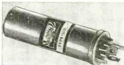
A special ventilating system allows internal gases to escape, but prevents air from entering, and a bakelite terminal base is used that completely eliminates leakage. Internal construction is all aluminum and electrolyte cannot come into contact with any corrosive metal.
