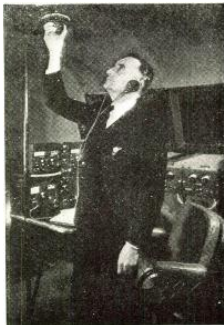
Atlantic Clipper planes spot their location by taking bearings on land radio stations.
