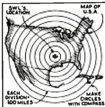
100 miles with the Amateurs or SWL's location as the center. The next circle will then have a radius of 200 miles, the next 300 miles, and so on until the map is covered. The circles can be marked as 100 miles, 200 miles, etc. Then the amateur or SWL can tell at a glance how far away the station to which he is listening is. I also have a map of the world fixed this way, with circles swung with a radius of every 1000 miles.—Kenneth Tyler.
