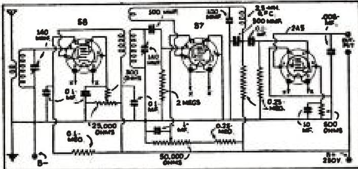
3-Tube receiver using 58, 57, and 2A5.
