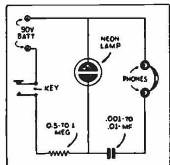
A Neon tube may be used to make the "code practice" oscillator shown above.
