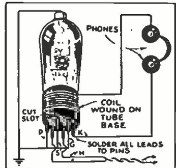
in length attached to one side of the coil, will aid considerably in picking up weak signals from the transmitter. Any type tube with a cathode may be used, and the filament of the tube is all that needs to be fed. Every phone man should have a monitor of this type in his shack.—W. R. Edelman.
