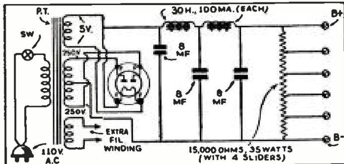
Power Supply Diagram for S-W Receivers
