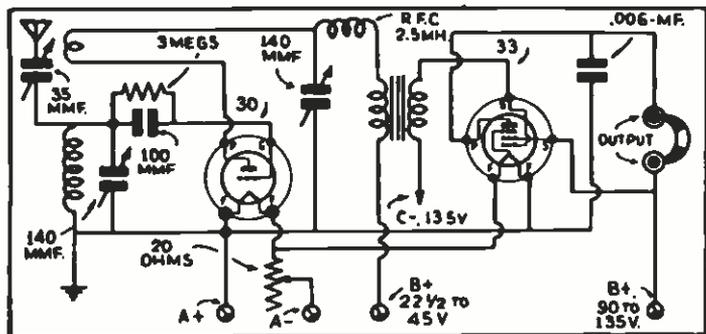
Two-Tube Battery set using a 30 and 33.
