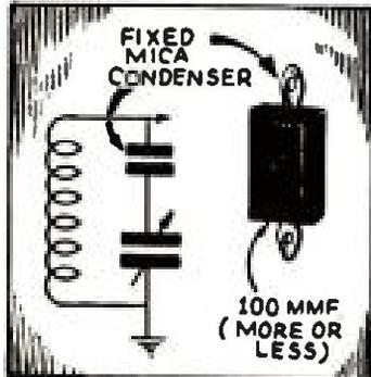
obtain better band-spread, and most conveniently too, by connecting a fixed mica condenser in series, usually about 100 mmf., with the stator. Thus, any variable condenser may be employed, even a 365 mmf. unit.—Eugelbert Bartoosh.
