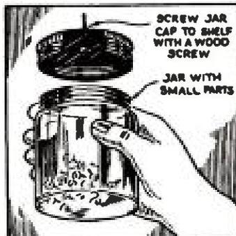
metal screw-top and fasten it to the underside of the shelf as shown in the drawing. In this way they're always kept in place and out of the way. —Eugene Poputs.
