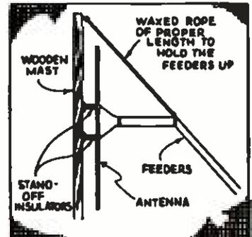
supporting the feeders to a two-wire matched impedance antenna of the vertical type. Those of us who have had any experience with such feeder systems know the difficulty of supporting the customary cross-arm on the vertical pole. The diagram will make clear the idea that I have in mind. Place the feeders exert a pull tangent to the mast, the rope is all that is necessary to insure against swinging. I trust that this idea will meet with your approval.—Maxwell Bittin, W9EN.
