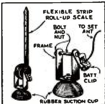
rolled up into a light, inconspicuous bundle. This is a particularly attractive feature for portable sets used out of doors. The drawing will illustrate the idea and its adaptability.—Ralph Scott.
