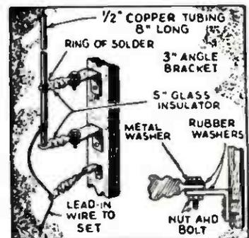
number of rubber washers cut from an inner tube. The 1/2 in. copper tubing may be too large to pass through the holes of the insulators; if such is the case, they should be filed to enable the tubing to pass through it. To prevent the tubing from sliding through the insulators a ring of solder should be placed above the top insulator.—Charles Zisk.
