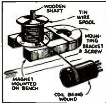
know will be appreciated by those radio experimenters who "wind their own" coils. Wind the coil wire on a tin spool and slip over a wooden shaft mounted between the poles of a magnet. This magnet provides perfect tension.—Ken Curry.
