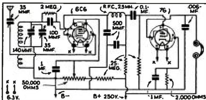
A "Ham" receiver, using a 6C6 and a 76. It has Band-spread and electron-coupling.
