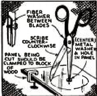
the material to be cut, then place suitable metal washer over point of narrow blade, insert in center hole and "scribe" bearing down on cutting blade. This works best with soft metals such as aluminum.—Walter Grossheim.
