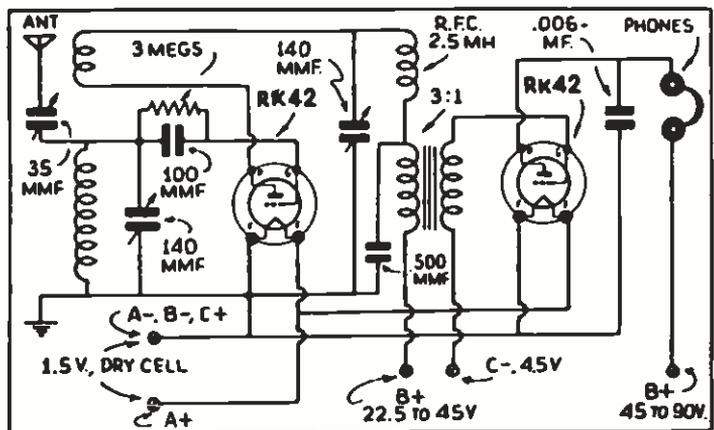
Battery Operated Receiver Using Low Drain Tubes
