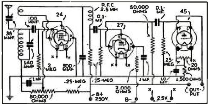
3 tube with type 45 output amplifier.
