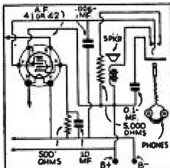
Diagram of the "Multi-Band 3" receiver shown in the May issue of Short Wave & Television. When the phone plug is inserted in the three-circuit jack (which is insulated from the chassis) it disconnects the speaker from the circuit and, at the same time, connects the 5,000 ohm resistance across the speaker terminals; and the 0.1 mf. condenser in series with the phones. I have built the "Multi-Band 3" and it surely works fine.—L. G. Saunders.
