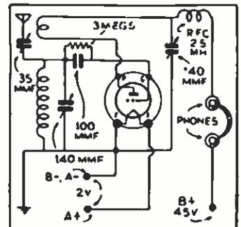
A 1-tube receiver using type 30.
