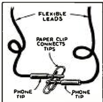
where temporary test connections are to be made. While the drawing shows two phone tips held together with a paper clip, almost any connection may be made in a similar manner. Flexible wires of course, as well as solid wires may be joined together without the trouble of twisting them.
