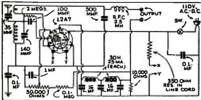
12A7 provides a 1-tube A.C.-D.C. receiver.
