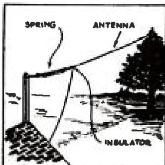
antenna wire and prevents breaking during a wind-storm when the tree usually swings considerably.—A. D. Margent.
