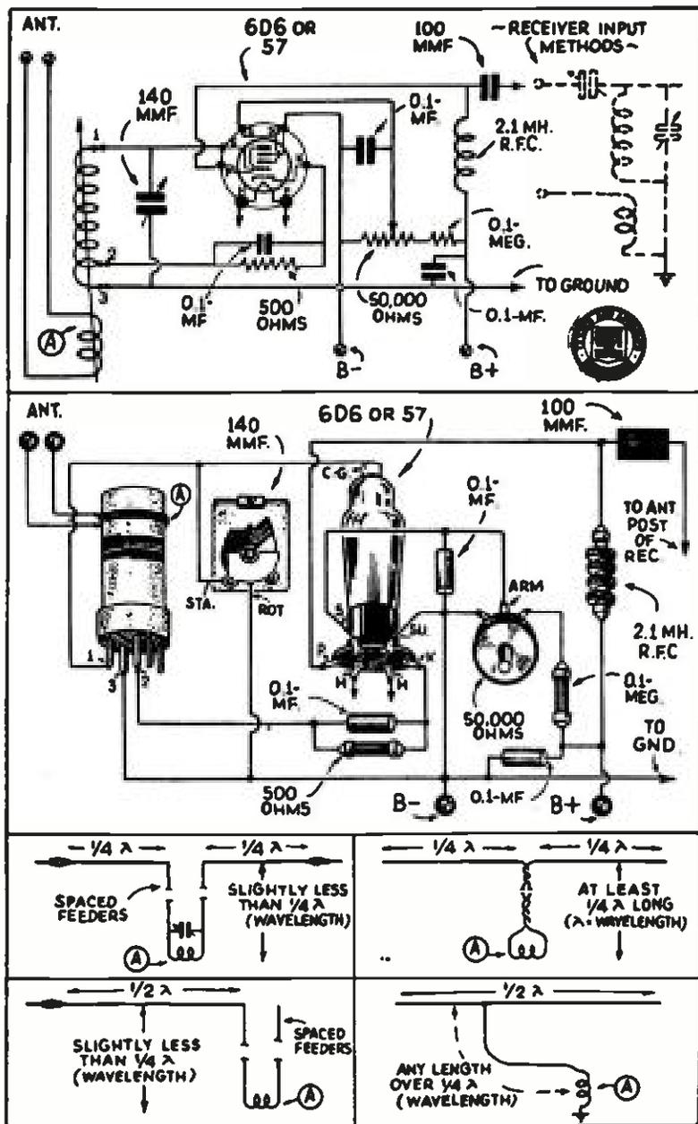
Diagram of pre-amplifier and improved antenna connections.
