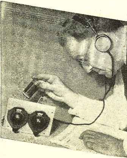
Changing bands on this single-tube receiver is a simple matter—just plug-in a different coil
