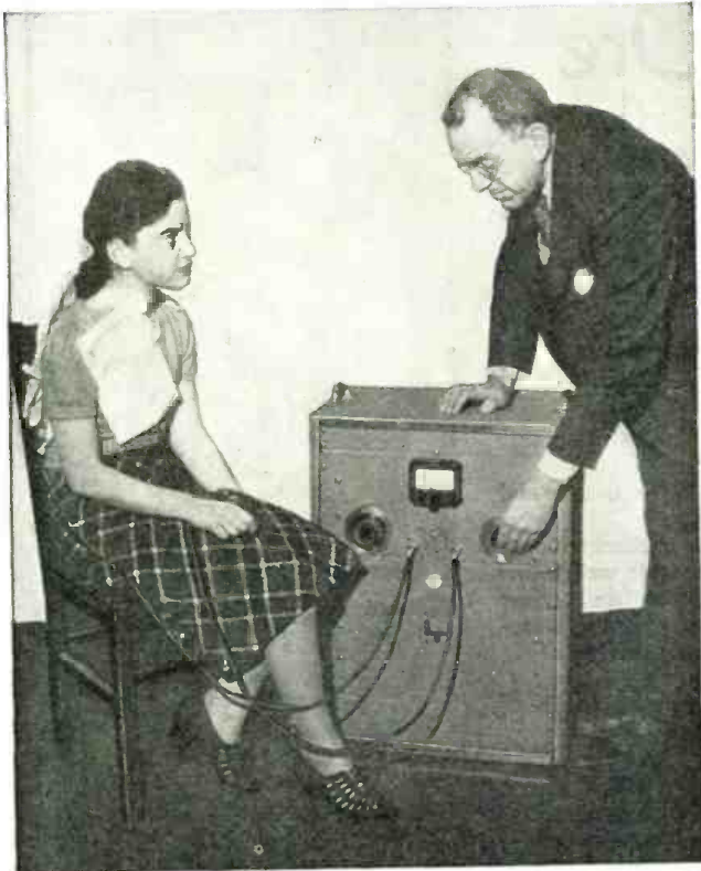
"Doc" Secor is here giving a treatment to a "patient." The electrodes shown are encased in washable cloth bags in order to absorb moisture. The left-hand knob controls the power output or "tuning," the right-hand knob is the 0-30 minute time switch.
