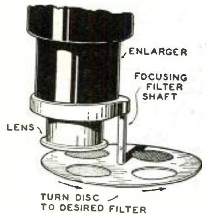
How filter disc mounts on enlarger.
