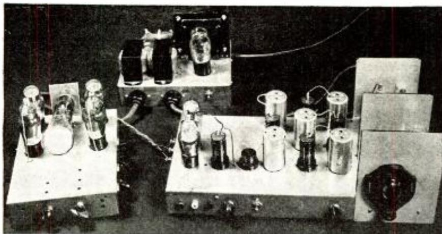
Fig. 2. Left—C-R tube and sweep oscillators; rear—power-supply; right—television receiver.
