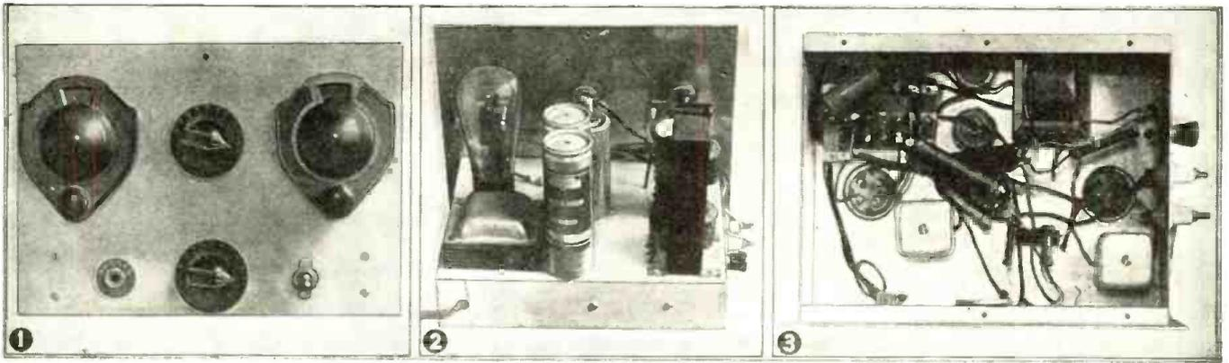
Photos show front, rear and bottom views of the 2-tube receiver.
