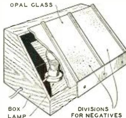
Construction of Comparator Box; standard negatives go in end frames, with new negative between them.
