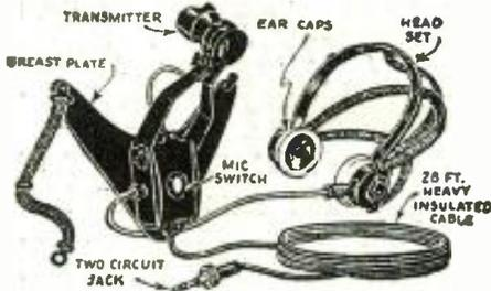
THIS Microphone and telephone headset outfit was built especially for the U. S. Navy Aviation Corps for Plane-to-Plane and Plane-to-Ground communication.
