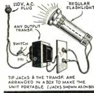
former, as shown in the accompanying sketch, as power for the flashlight used to inspect receivers in my service shop. Any output transformer will provide the low voltage high current necessary for flashlight bulb operation or, if one prefers, a filament transformer can be used, in which event standard pilot light bulbs can be operated in the flashlight at their normal brilliancy. And it's always ready when needed.—A. Morino.
