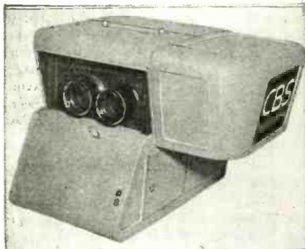
Here is CBS's latest television studio camera. It incorporates a number of special features, including a non-inverting view-finder, minimum parallax and a newly designed head-amplifier.
