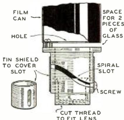
How focus slot is made light-tight.
