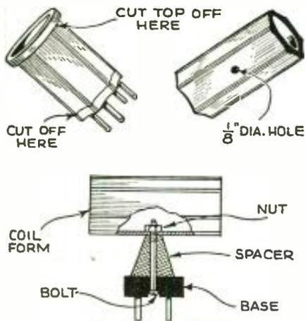
the two parts together using the upper half of a "pee-wee" feed through insulator as a spacer. The coil must be taken apart before the wire can be wound on it and when this is done one-half inch should be left between the two windings to accommodate the top of the spacer. This type of coil is very convenient in many applications and will not cost much more than 25 cents.—E. J. Rohrig.
