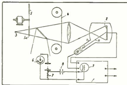
film "for a time equal to the previous stoppage and such a number of times that the beginnings of two successive stoppages are separated by the duration of a scanning of the photoelectric surface, and continuously scanning the screen while the film is projected and while it is obturated."
