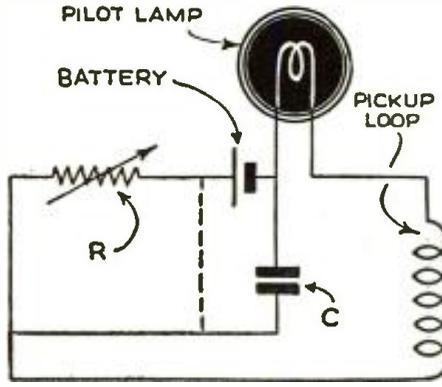
energy will increase its brilliance from dull red to dazzling white. The 70% of the energy is supplied by a small battery and variable resistor in series with the bulb and coil as shown in the diagram. Resistor R is adjusted until the bulb glows dull red. Condenser C may be any small condenser which is available. The pickup coil is now loosely coupled to the transmitter circuit. If a two volt .06 amp. pilot bulb is used, no
