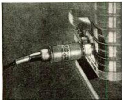
only high impedance input circuits. This handy piece of apparatus which connects between the microphone cable and the amplifier input connection is available in two types. One provides for voice coil connection of dynamic mikes, as it has a primary impedance of 30 to 50 ohms; the other is a 200 to 250 ohm unit for dynamic or velocity mikes which have self-contained line output transformers. Both types are magnetically shielded to reduce hum pickup. Mfd. by Thordarson.
