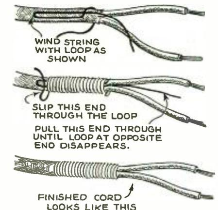
ping as possible. The cord will be firmly secured, and no knots or loose ends will remain.—Steve Liska.
