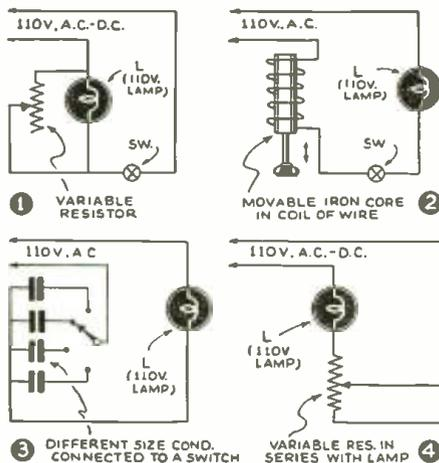
If you have a number of condensers of different capacity lying about, several of these may be connected to a switch as shown at Fig. 3; the lamp will light the brightest on the large size condensers, and dimmer on the smaller capacity condensers. One of the usual ways of dimming a lamp is to connect a variable resistance in series with it as shown in Fig. 4.
