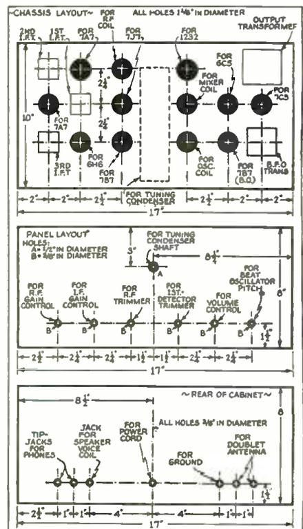
Above—Chassis and front panel drilling dimensions.
