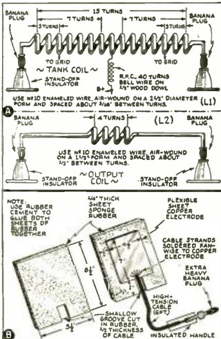
Details of short-wave diathermy coils, also construction of treatment pads. (No. 1228)
