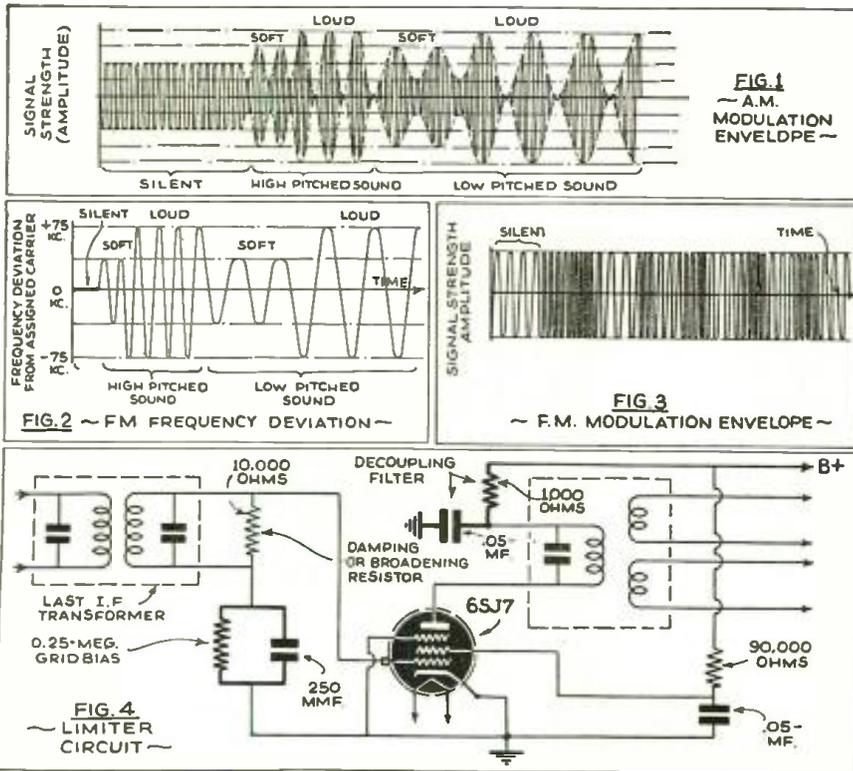
The difference between frequency and amplitude modulation is readily apparent by looking at the graphs.
