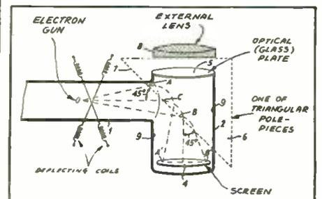
The cathode ray is bent at right angles.
