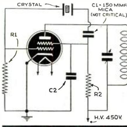
was used, depending on the available heater voltage. I have used 450 to 500 volts on the 6L6G without experiencing any trouble and any type of crystal will oscillate in this circuit. The power output is very good and the note steady.—*Allan Ford, VE2PF.*
