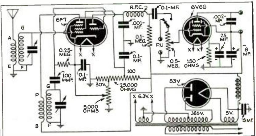
Simple phono pickup and 2-tube amplifier; right—useful radio tuner unit which can be added ahead of the phono unit.
