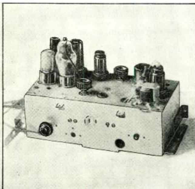
Photos show external appearance of the special radio receiver which operates on waves radiated from automobile engine; chassis at right.
