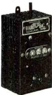
• AN improved and very compact Wireless Phonograph Oscillator has recently been announced by Bud Radio, Inc. This unit is primarily intended to adapt standard wired record players for wireless operation with a minimum of effort and expense. Measuring only 4 1/2" x 2 1/2" x 2", the oscillator may be attached inside the case of most record players, thereby eliminating the usual nuisance of unsightly external apparatus and wiring.
