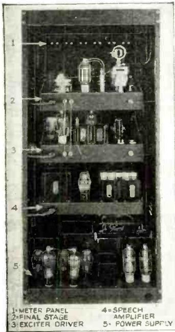
← Rear view of complete transmitter—Power supply is built-in at bottom of cabinet.
