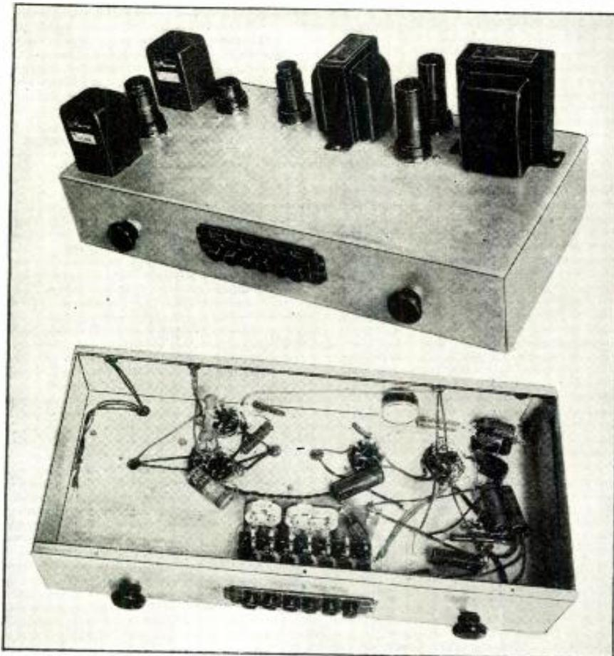
Front view, showing the placement of the tubes and transformers. The under-chassis view illustrates the extreme simplicity of the wiring.
