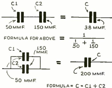
NOTE: WHEN USING FORMULAS ALL CAPACITIES SHOULD BE GIVEN IN THE SAME UNIT (EITHER MF. OR MMF)
