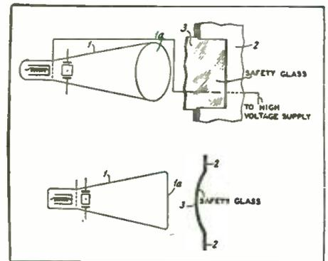
If the protective glass breaks the high voltage circuit to the C-R tube is opened.
