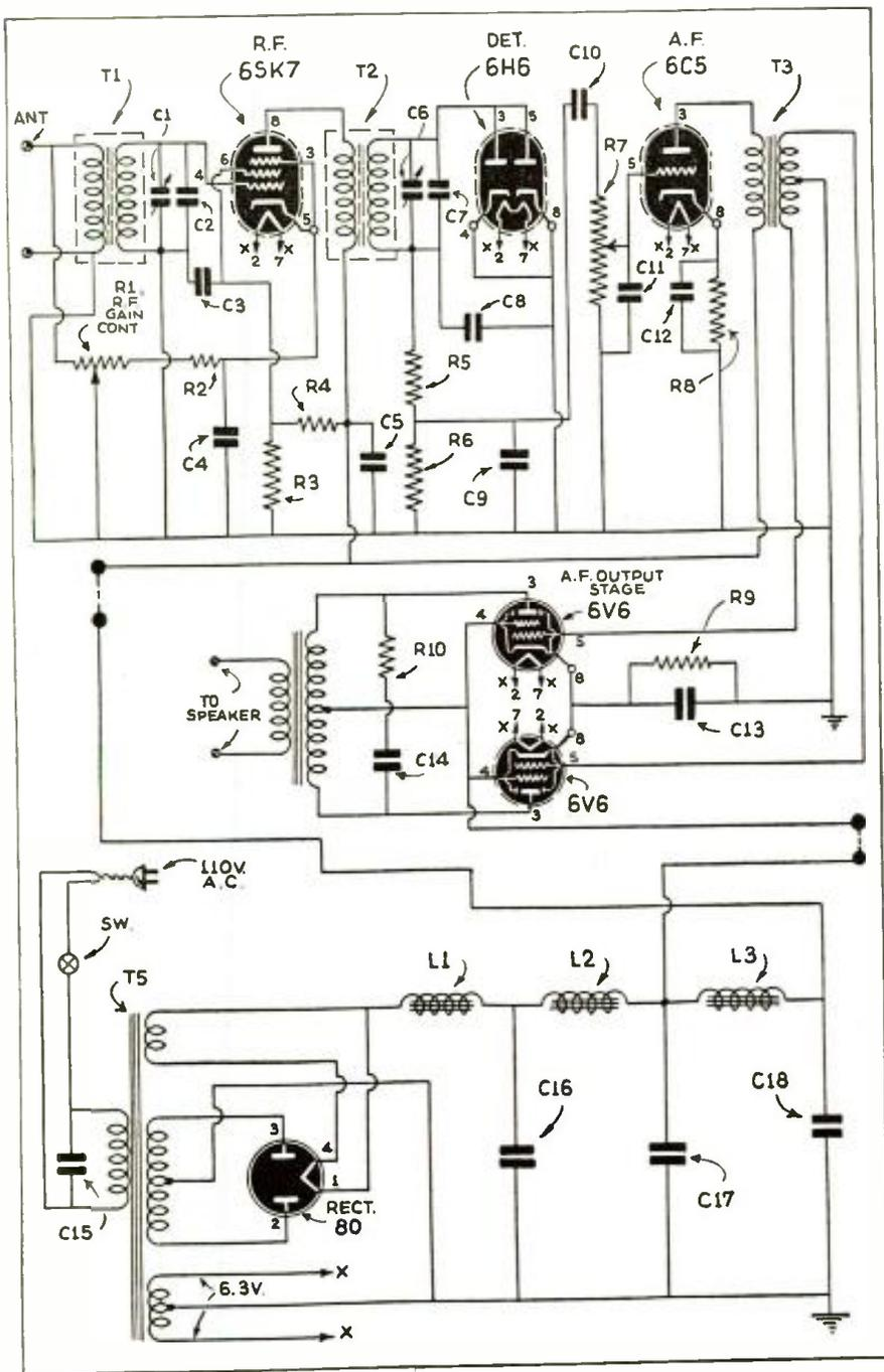
The diagram makes it apparent that the construction of this BC set is simplicity itself.
