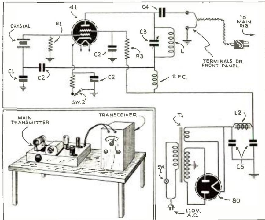
How old transceiver was re-wired to make plug-in oscillator.
