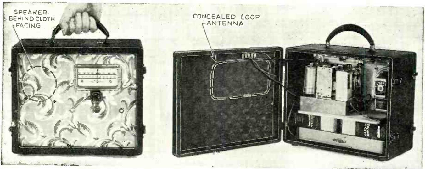
Left—Front view of 4-tube portable: right—rear view with lid open, showing batteries.
