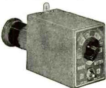
and condenser combination together with a suitable pilot bulb for resonance indication, and band switching is employed enabling the unit to cover all amateur bands from 10 to 160 meters. Calibration is indicated on an etched nameplate, and the case of the unit is finished in attractive Grey Crackle.
