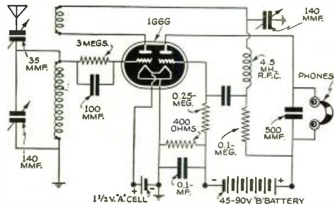
One tube does the work of two in the "Twinplex." (No. 1229)
