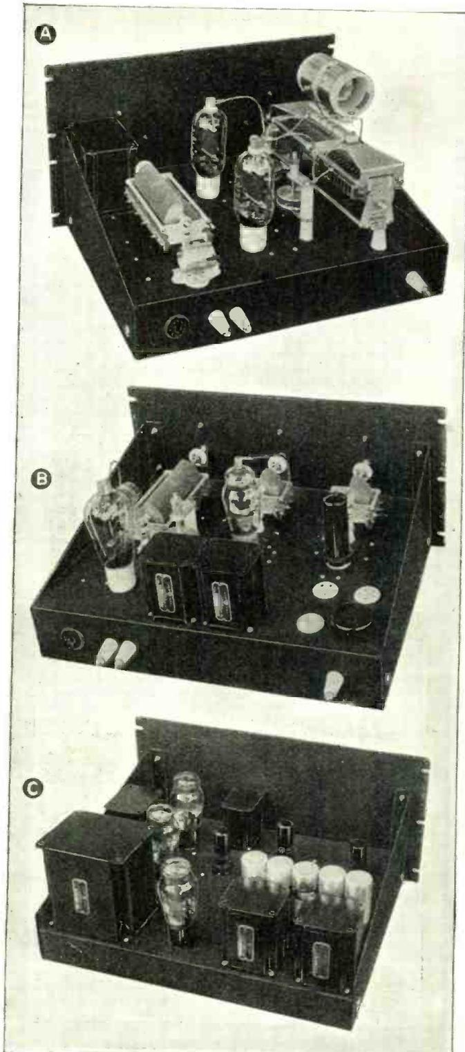
Left—Rear views of respectively Final Stage; Exciter-Driver Stage, and Speech-Amplifier unit.
