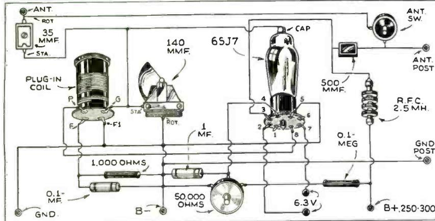
The general appearance and also the simple wiring diagram to be followed in building the preamplifier are here illustrated.
