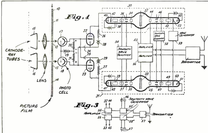
In this television system only the differential signal is transmitted; thus a narrower frequency band may be used.
