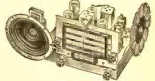
Television and FM adapter connections. Tuning range for standard broadcasts is 535 to 1,720 kc., and 5.65 to 18.3 mc. for foreign and domestic short-wave. Uses latest multi-purpose tubes: 12A8GT, 12J5GT, 12K7GT, 12Q7GT, 35L6GT, and 35Z5GT. Employs a 6 1/2" FM dynamic-type speaker for realistic reproduction.
