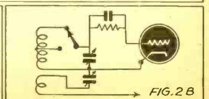
single coil with a tap on it. If two separate coils are used, separate tickler coils should preferably be employed which requires a separate switch just for the tickler coils alone.
