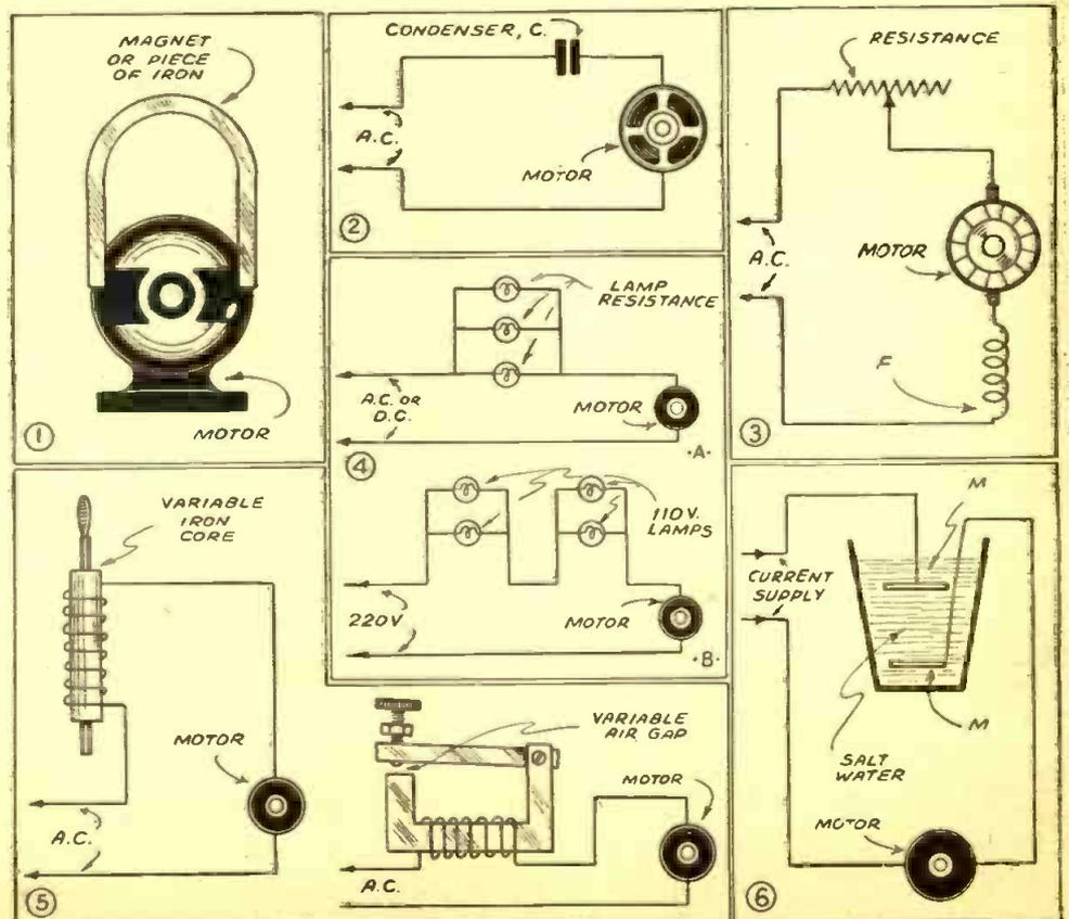
connected in series with a motor to regulate its speed. Various speeds below normal value may be obtained in this way. Salt water is used in the tank, which may be a wooden barrel or pail and two metal plates M-M are submerged in the solution, the top plate being movable up or down, so as to vary the distance between the two plates and thus regulate the amount of resistance in series with the motor.
