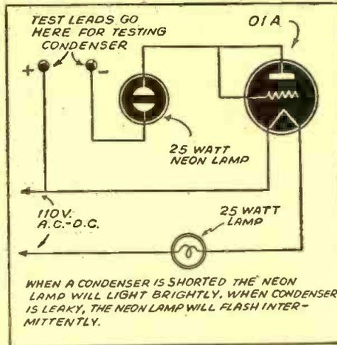
The diagram above shows a simple condenser tester contributed by Leon A. Wortman, W2LJU. This device will quickly indicate defective condensers. Be sure to observe polarity on electrolytic condensers.
