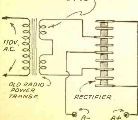
power transformer and a dry disc rectifier of the Elkon type M-16. A little experimenting may be necessary to get the filament windings of the transformer connected in series so as to get the desired voltage. The output of this charger is from two to four amperes at six volts. For those having an old "A" battery eliminator of the dry rectifier type, they may have an efficient charger by removing all resistance, chokes, etc., and connecting the battery to the output.—H. D. Malvin.
