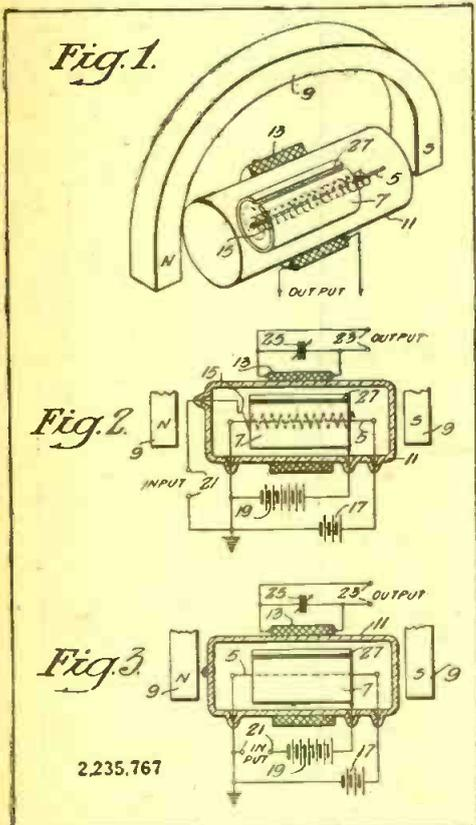
Note use of magnet to control electron stream.
