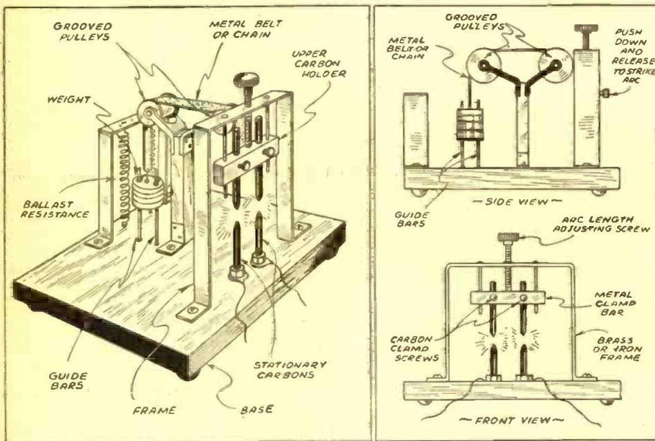
Simple design of home-made arc, suitable for "sun-tan" treatments, etc.
