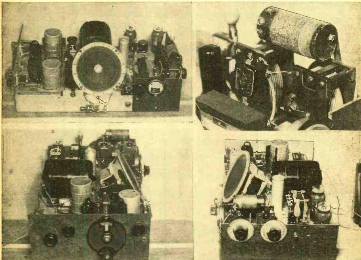
Various views of the portable phone transmitter and receiver, made mostly from odd parts found about the Ham shack.
