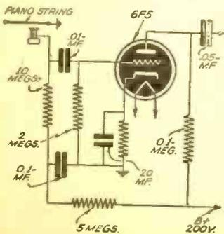
Electrostatic pickup under string of instruments. (No. 1256.)
