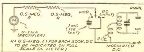
This simple circuit, together with an ordinary meter, will be found extremely useful by the amateur to check modulation and voltage.
