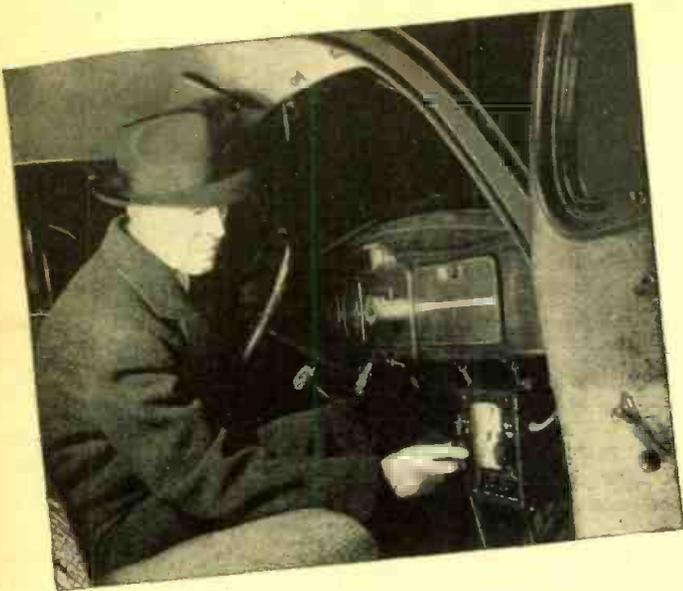
The mounting accessories consist of two self-threading hooks turned into the dash, and a metal strip bolted to the engine bulkhead. A stud or projecting bolt-head at the bottom edge of the receiver locks into the keyhole-shaped hole on the foot of this strip. Screw-eyes in the front-top of the receiver slip into the dash hooks. The "S" hooks provide an extension to clear the handle atop the receiver.
