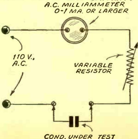
obtain a "zero-adjustment" on the meter. Since the circuit is essentially a series circuit, with the condenser test leads shorted a full scale reading should be obtained. An open condenser (shorted condenser) will give a full scale reading while a good condenser will give a reading proportionate to its capacity.
