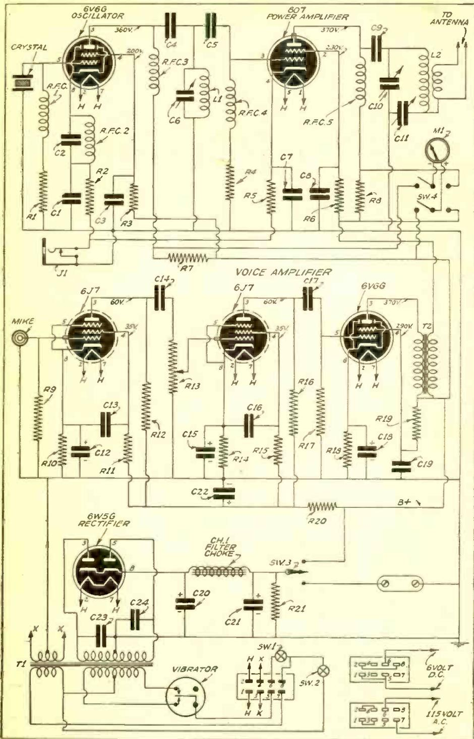
Above—Diagram of the 12-watt phone or CW transmitter.
