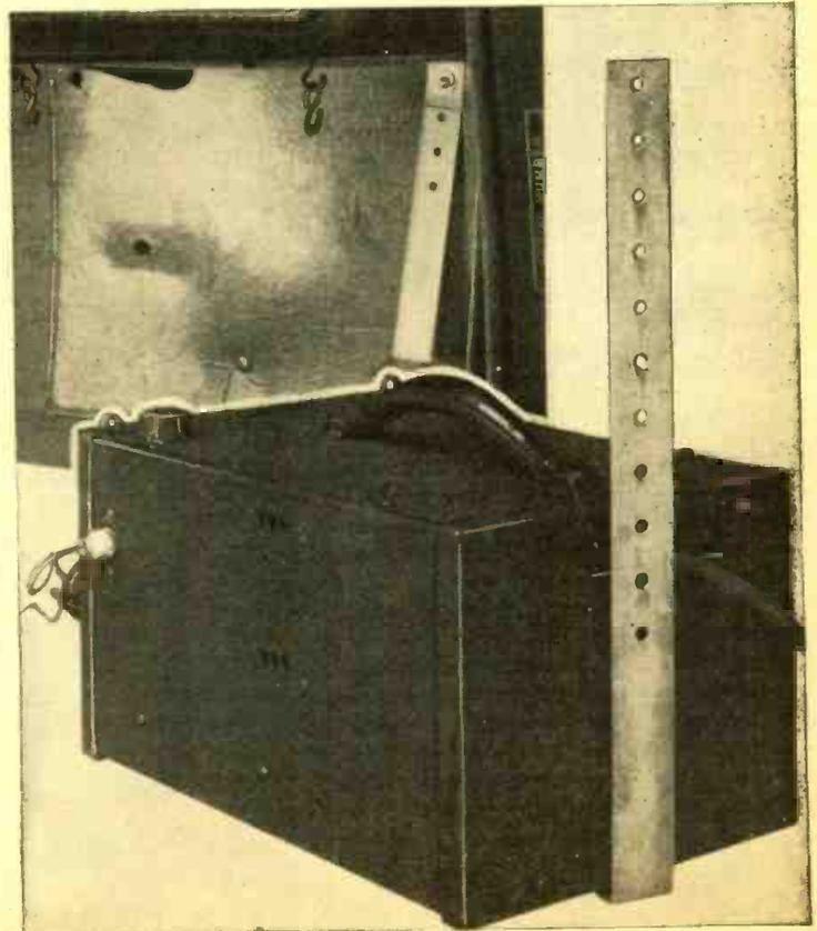
The S-29, showing screw-eyes and mounting strip. This strip is permanently installed on the engine bulkhead. This receiver suggests two other convenient features for portables—the compartment at the rear to accommodate the line cord when operating from self-contained batteries, and the "plug-in" antenna arrangement.
