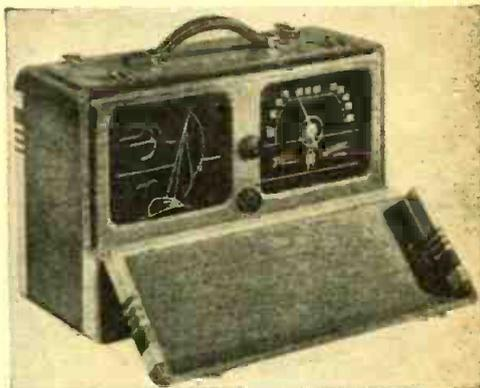
The handsome portable receiver (Model 6G601M) here shown is awarded to Eldred Winn for his editorial. This is a three-way portable and operates on 110 volts A.C. or D.C. and also on self-contained battery. The set uses six tubes and is enclosed in a handsome portable case, with a hinged lid which protects the dial when it is folded in the closed position.
