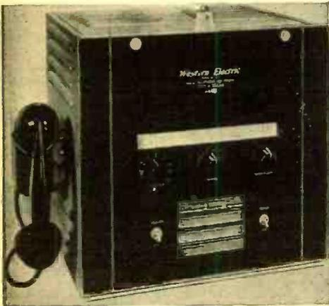
A single control is provided in the 226-D for shifting both the transmitter and receiver simultaneously to any one of ten frequencies. Nine of these may be utilized for ship-to-shore communication and the tenth reserved for ship-to-ship or coast guard. All controls are located on the front panel, where they easily may be reached.
