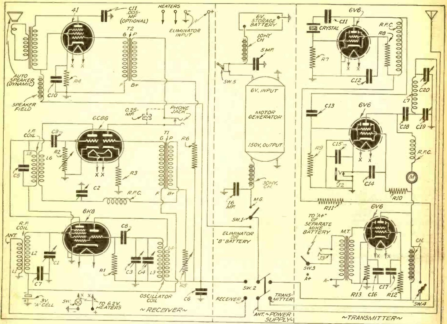
Complete wiring diagram of the low-power portable transmitter-receiver.
