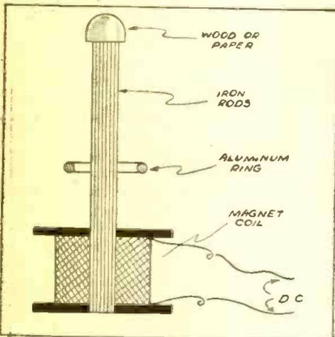
The aluminum ring jumps upward each time the current is passed through the coil.
