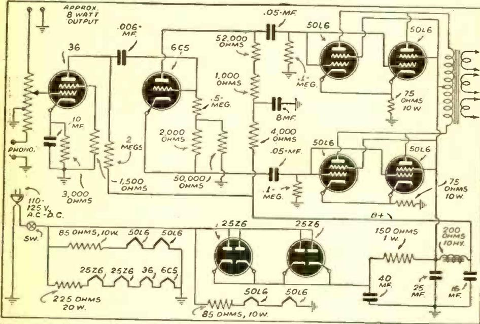
Rex C. Dudoward provides this interesting circuit of an audio amplifier, using four 50L6 tubes in the output stage. He suggests that the 36 tube be changed to a 6J7 or 6SF5. The output transformer should have a 3,000 ohm primary center tap, capable of passing 100 ma. All resistors are one-half watt unless marked otherwise.
