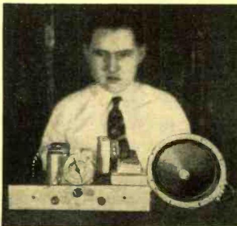
A front view of the T.R.F. 7 broadcast receiver with loudspeaker. It may be mounted in a suitable cabinet and the tone quality improved by a suitable baffle chamber.
