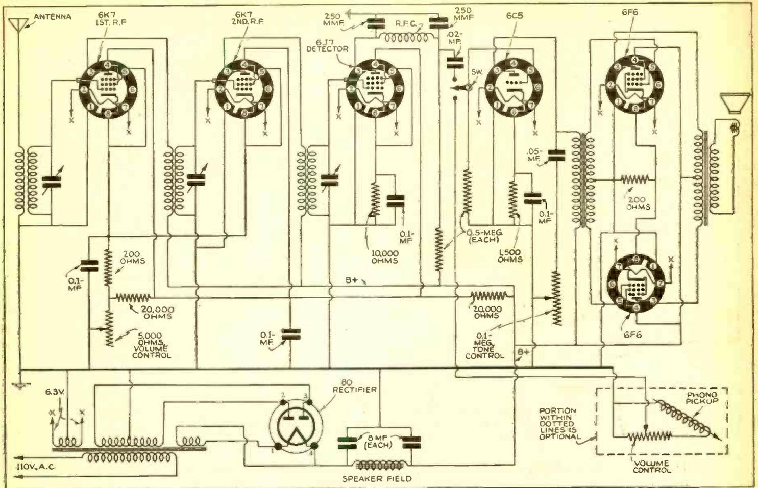
Wiring diagram for building the T.R.F. 7—a T.R.F. receiver with plenty of pep!
