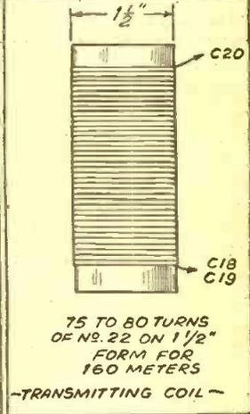
Auxiliary diagrams showing plan of layout of "transmitter-receiver," together with coil winding data.
