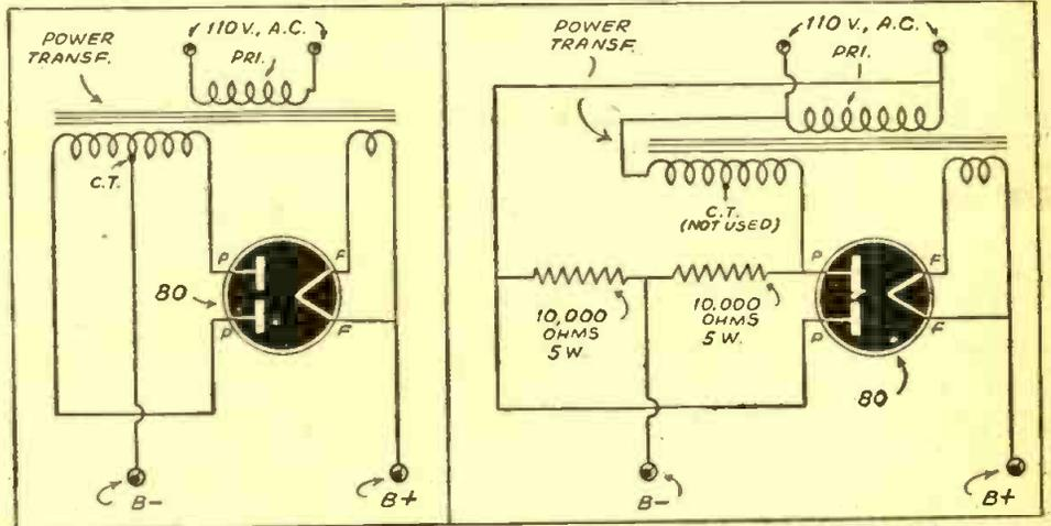
Edgar Boles contributes the above circuit for increasing the voltage of a power-supply; standard circuit at left and revised circuit at right. Transformer primary is connected as auto-transformer, making the voltages additive. Use condenser in series with "receiving set" ground.
