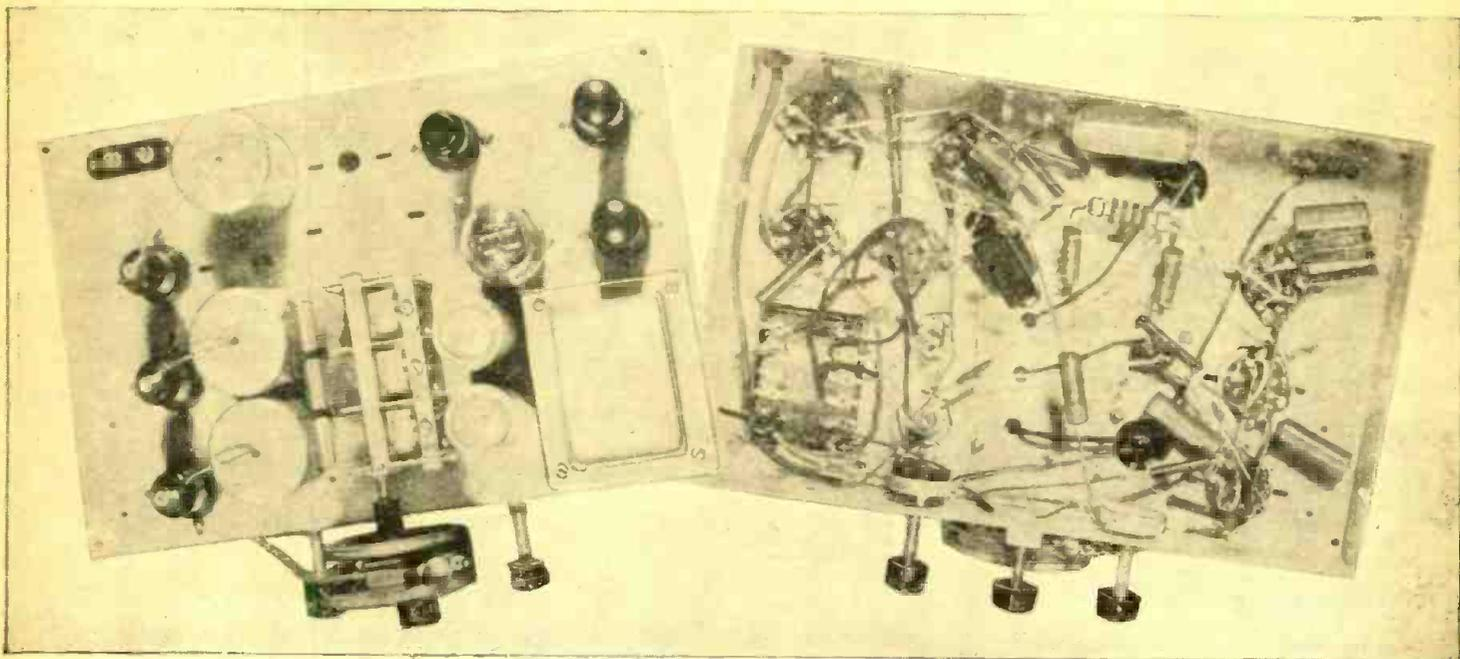
Top and bottom views of the T.R.F. 7—a tuned radio frequency receiver for the broadcast band.
