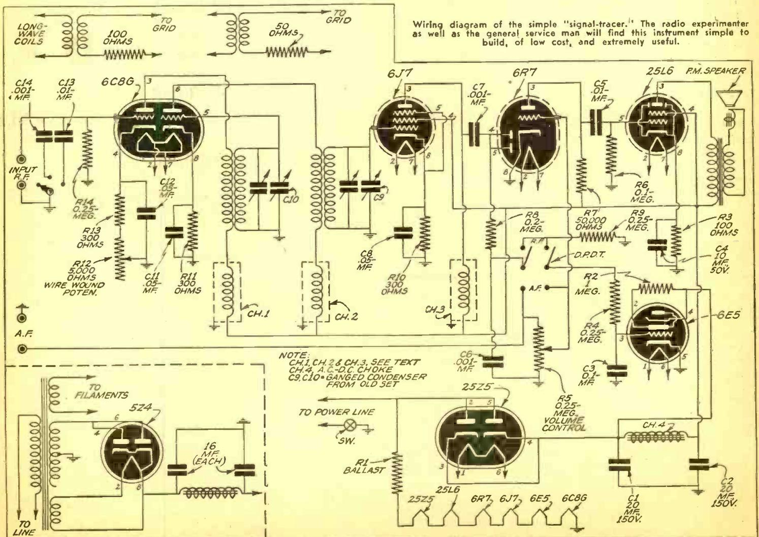
cautions aren't taken the signal-tracer and the receiver under test may be grounded on opposite sides of the line, and "fire-works" and blown fuses will result. As it is, it is necessary to always *ground* the tracer to the receiver under test, to form a proper path for the signal and to prevent hum.
