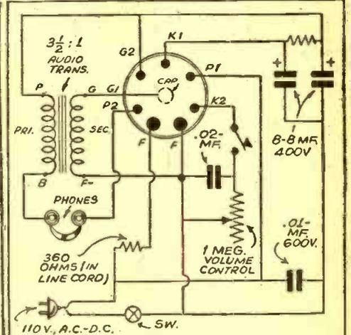
Gene Clardy sends this diagram for a simple code oscillator, made of odd parts found about the shack. The volume control serves to vary the tone. A 12A7 was used by the author.
