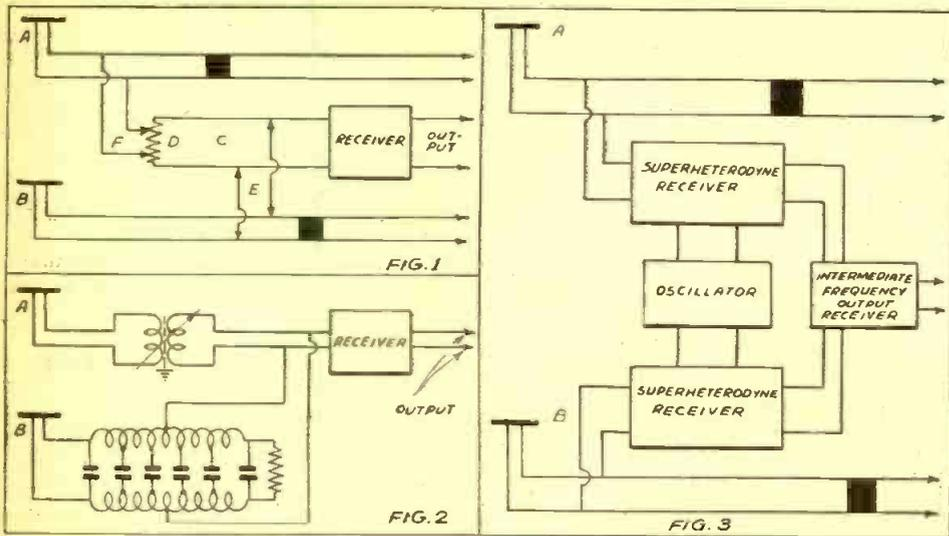
● RECEIVING antenna for ultra short wave use which shall be comparatively free from the effects of man-made static
