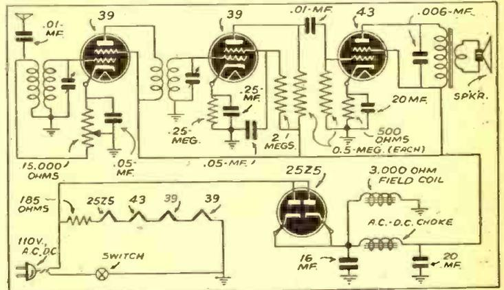
Diagram for 4-tube Broadcast receiver. (No. 1255.)
