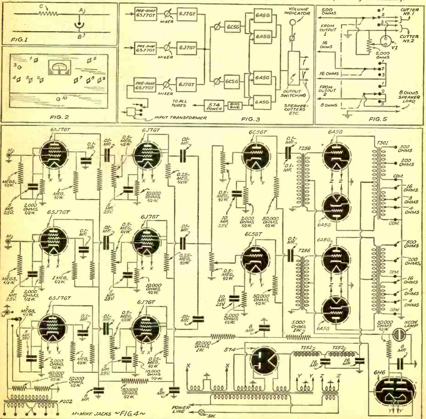
indicator. The DB meter may be calibrated against the Class B plate milliammeter or better yet against an oscilloscope. This operation is quite simple. A calibration chart is drawn up showing at what point on the meter 100% modulation is shown on the scope. These percentages may be recorded from 0 to 100 in whatever steps the operator desires, although 0, 25, and 100 should be ample.
