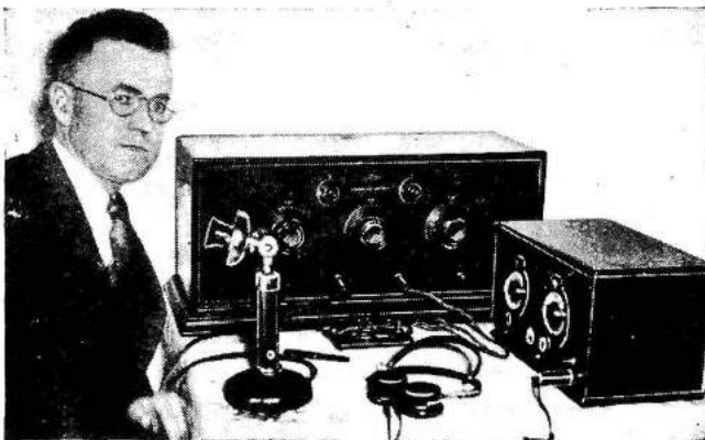
The author with his transmitter constructed from an old neutrodyne receiver.
