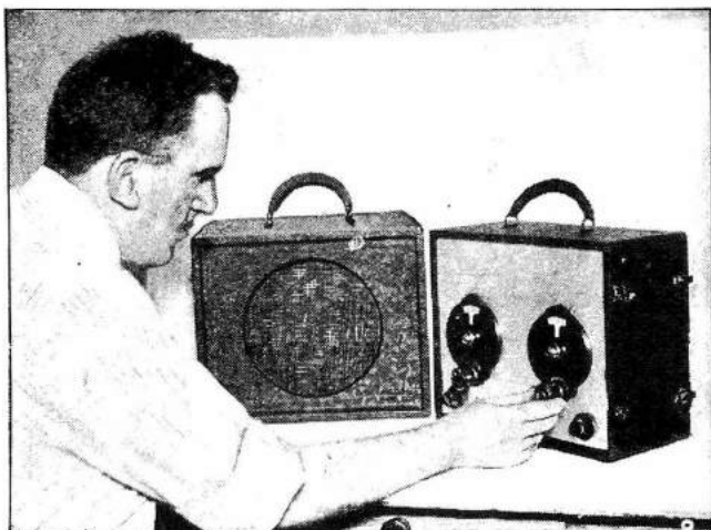
H. W. Secor is here shown trying out the 8-Tube Portable "All-Wave" Superhet designed by Mr. Denton.
