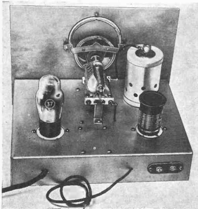
Directly above, we see the single-stage R.F. booster connected to a Midget all-wave receiver (right).
