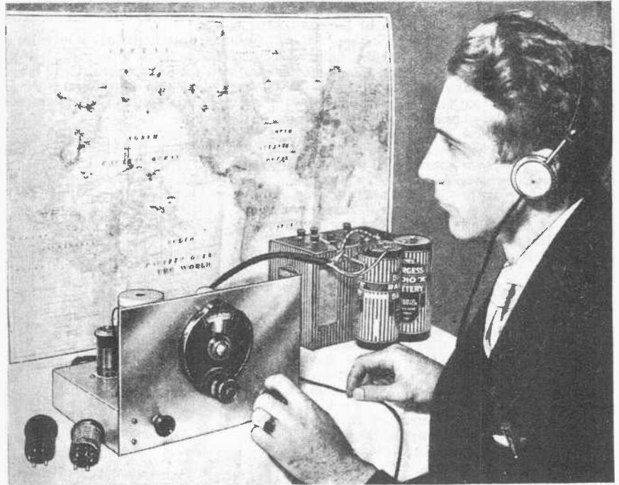
The designer of the "3-tube equals 5" Battery Receiver, which features the use of a separate regeneration triode, is here shown giving the set its final test. "O.K." says W2AMN.
