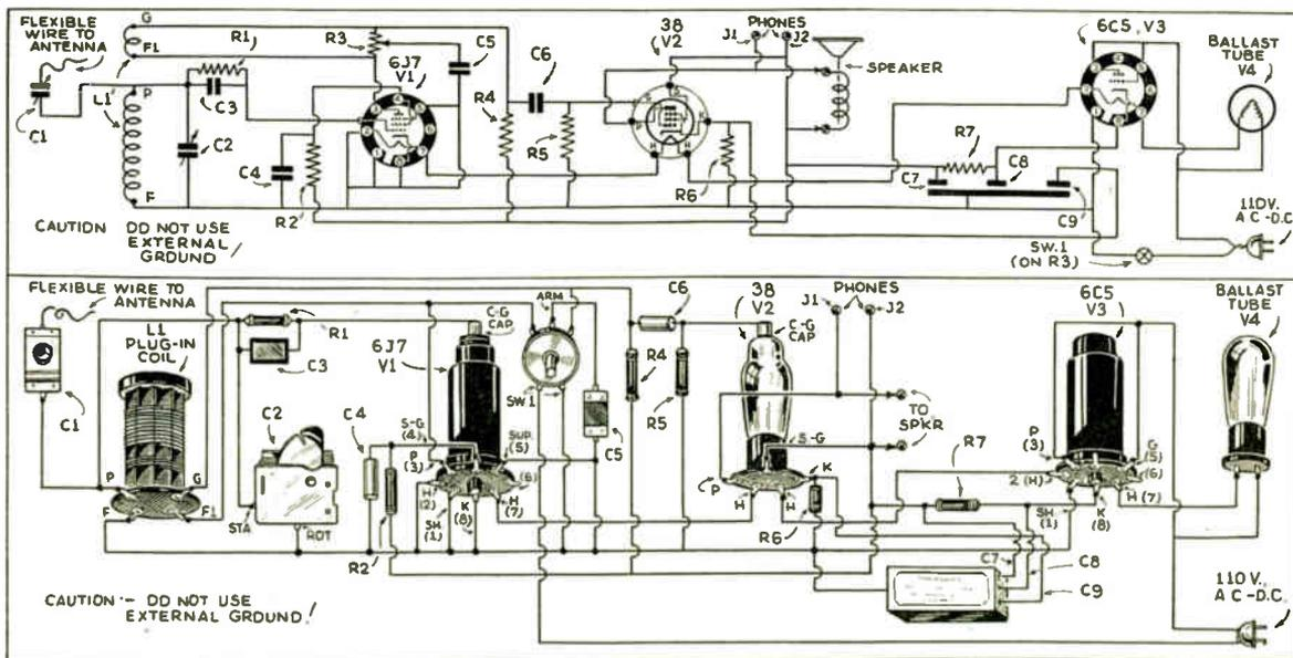
Wiring diagram for the Jr. "Space-Explorer"
