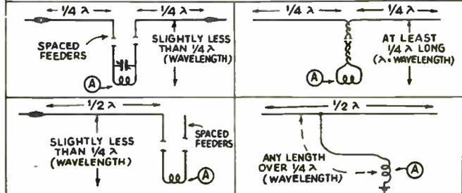
Diagram of pre-amplifier and improved antenna connections.
