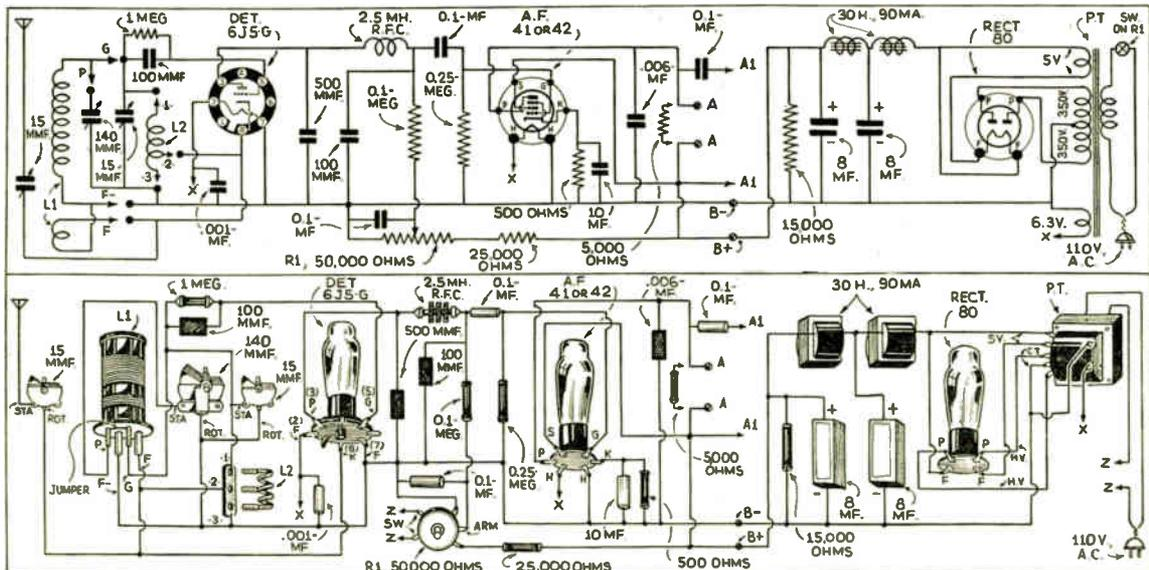
Wiring diagram of the "multi-band 2" receiver. The tubes selected for this set ensure the maximum results.
