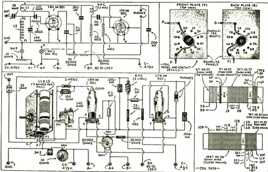
Fig. 1. Complete wiring diagrams both in schematic and picture form are given above for the 2-volt receiver.
