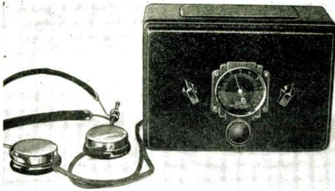
*A 2-Tube the S-W "Fan" has been waiting for. It operates on batteries. Simple switch enables operator to change instantly from one band to another. Range 16 to 550 meters.*
