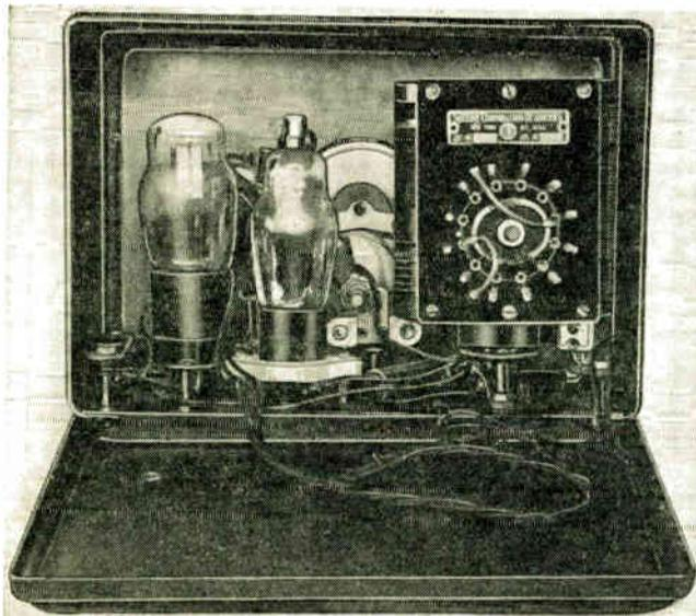
Photo above shows a rear view of the 2-volt receiver, which covers 16 to 550 meters with a handy band-switch
