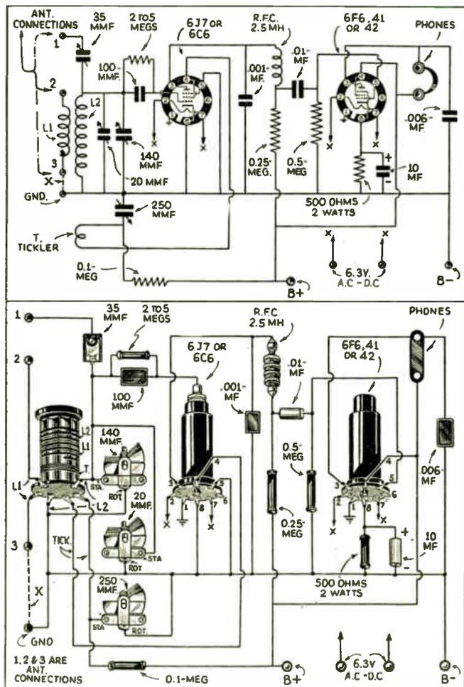
Fig. 1. Hook-up of 2 tube regeneration receiver.
