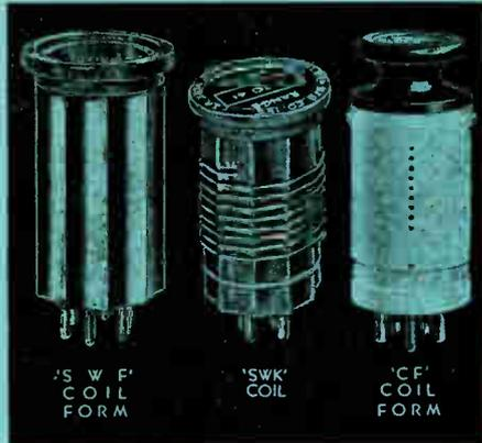
"SWK" coil kits, two- and three-windings, are bound to give better reception. Wound on XP-53 low-loss material they just fit the receivers described in this book. "SWF" and "CF" are blank coil forms.
