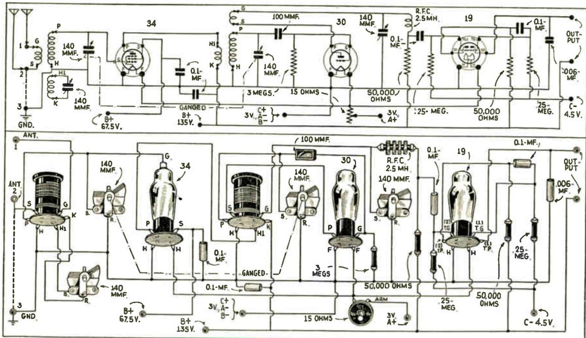
This diagram very clearly shows how to wire the improved battery-operated Doerle receiver.
