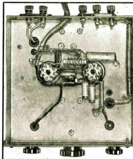
is almost doubled over that for a single tube—as can be at least fairly well shown with the pre-selector in operation, by lifting one grid cap connector from tube contact and noticing the drop in signal level.
