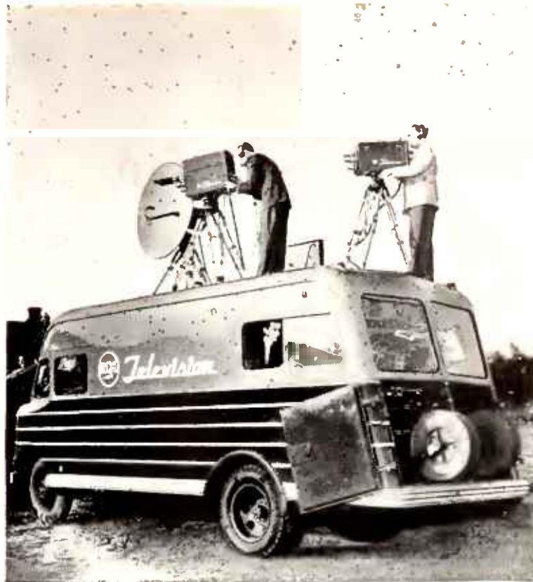
Mobile television van operating “in the field”—note complete camera facilities, and microwave relay apparatus.
