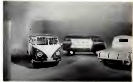
1. Vehicles are filmed against all-blue background on Eastman color negative film which can filter out any of its three primary colors
