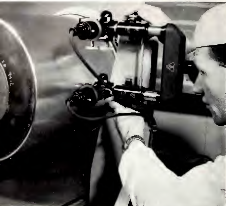
Xerographic drum surface is inspected by comparison microscope to insure flawless uniformity required for high-quality copying.
