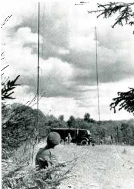
Mobile radio transmitter BLA-3, "the little broadcasting studio on wheels". The masts, almost 100 feet high, were erected in a matter of minutes.
