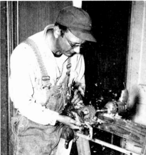
You've heard about Warren Neilson's duck picking machine, and here it is, with the feathers flying. It is a rubber buffer on a steel bit which he mounts on an electric drill. Warren has been duck hunting at every opportunity and so far has kept the picker busy. The buffer gets most of the feathers in short order. Warren then dips the duck in paraffin, allows it to cool, and peels off the pin feathers. Certainly a slick operation.
