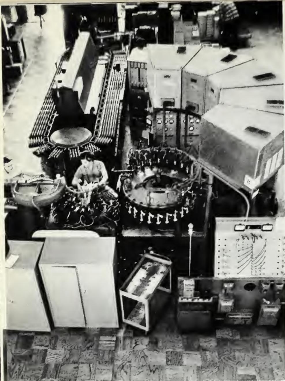
*Vacuum tube assembly involves automatic machine aids, but key processes are in human hands of extraordinary dexterity. ABOVE: Sealed vacuum tubes are fed at high speed to conveyor belt. BELOW: Nimble fingers skilfully, speedily assemble tiny tube parts.*
