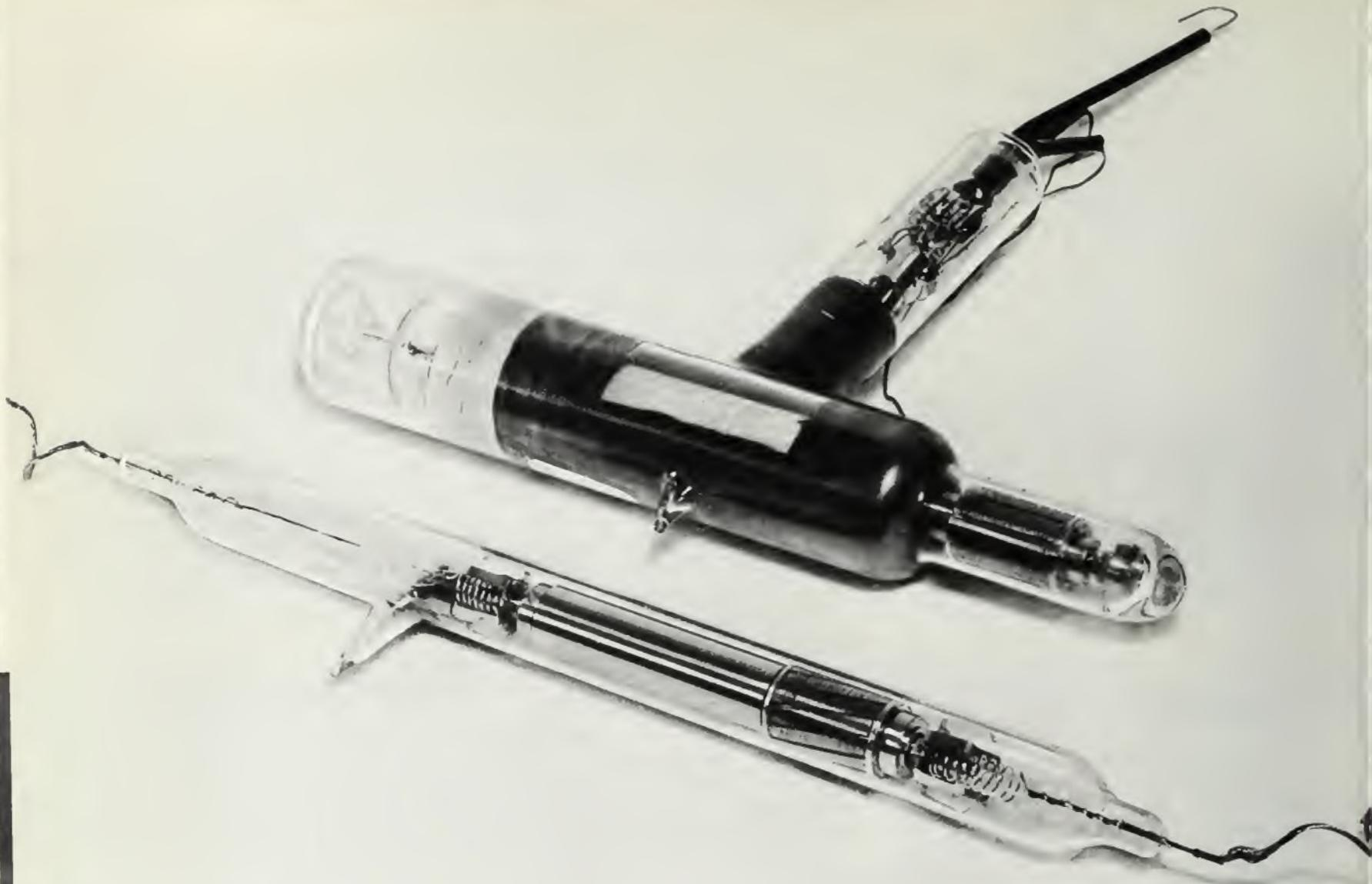
*ABOVE: Special equipment for testing CBS Laboratories-developed low-friction vacuum bearings for use in high vacuum, as in outer space. The new bearings extend very substantially the effective life of instruments that operate in a high vacuum.*
