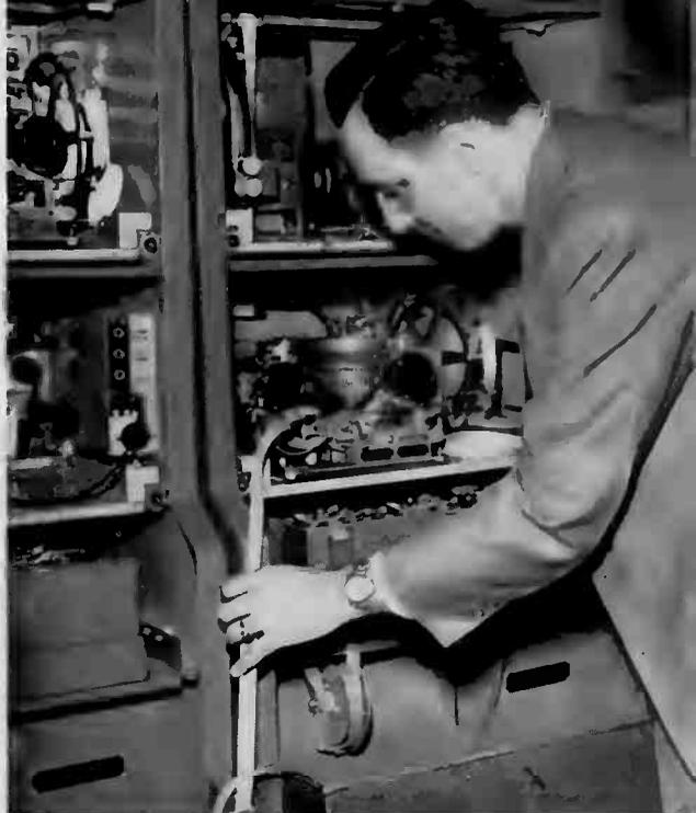
**Automatic transmitting and receiving equipment is combined in one compact unit. Bottom section of unit contains sending equipment; center section, receiving equipment; top section, monitoring equipment.**
