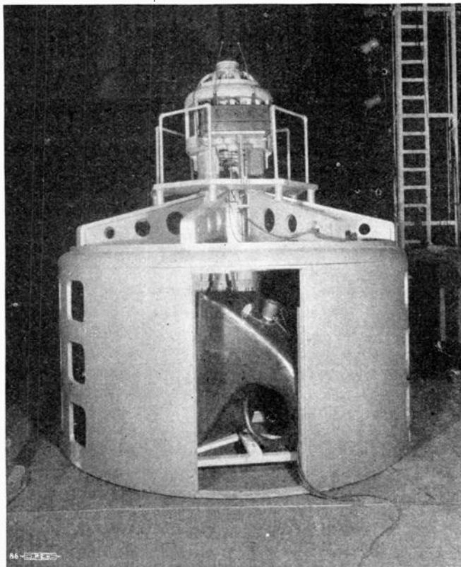
View of Amplion giant dynamic and exponential horn mounted within dynamo on stage
