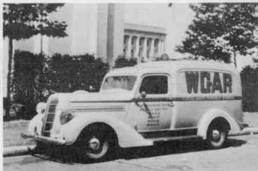
The WGAR Mobile Unit No. 1—housing special short wave equipment which can be transported to the scene of any activity so that broadcasts can originate at that point.
