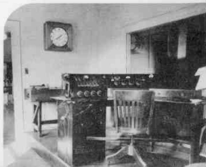
The master control console in WGAR's Hotel Statler studios. From this point all programs are "monitored" to be delivered to listeners with the greatest degree of tone realism.
