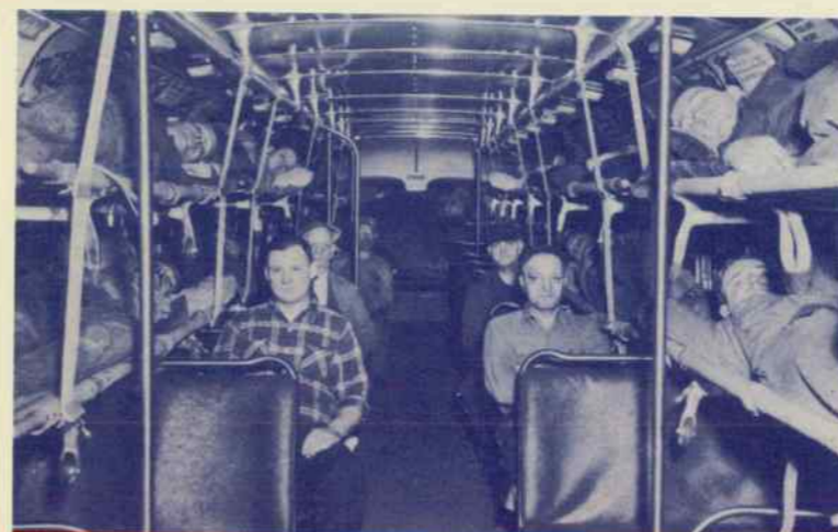
A graphic demonstration showing how Cleveland CTS buses can be rapidly converted for the handling of casualties in the event of a disaster.
