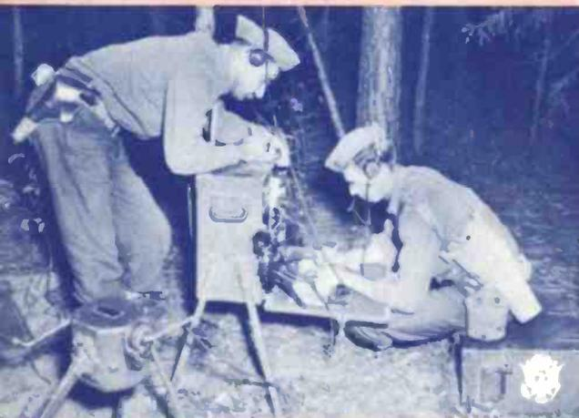
Portable Army radio outfit operates on maneuvers. Note hand generator.
