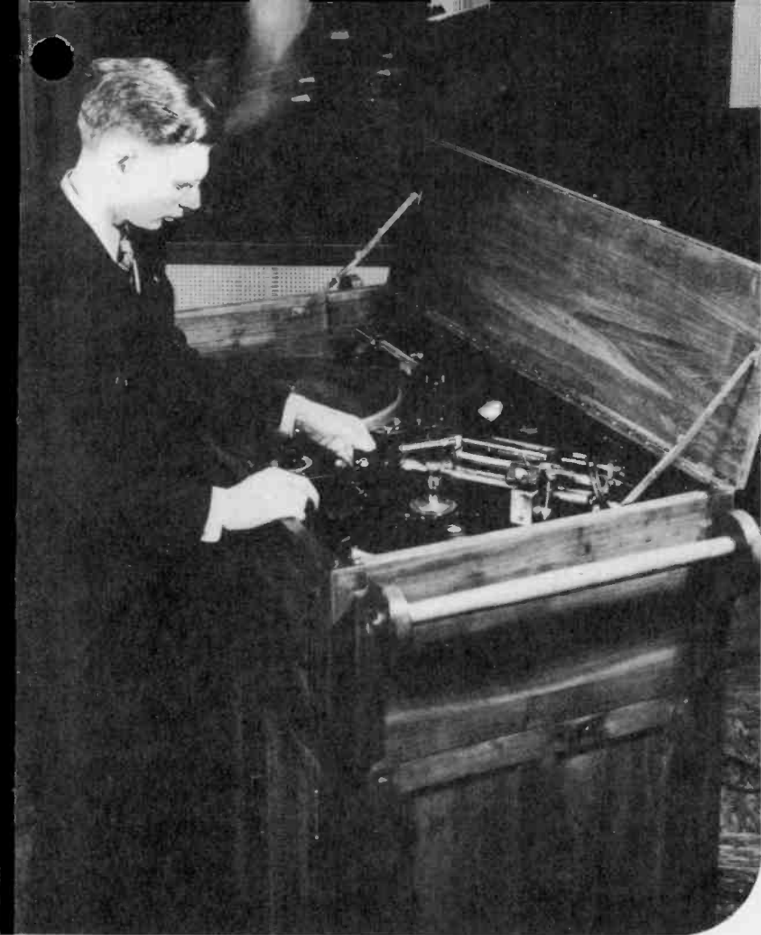
Another innovation credited to the WKBN technical staff is this compact "sound effects wagon." It is so constructed that it may be used to cut or record transcriptions; can be quickly altered to "play back" for audition purposes; can be connected to play transcriptions for broadcast, or can be used to introduce recorded sound effects during studio dramatic presentations. Its specially designed undercarriage also permits its easy transfer from one studio to another. Engineer Carl Lindberg is shown at the unusual machine.
