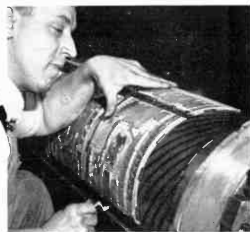
ED FRANK, one of pressmen, locks electrotype plate onto a cylinder of the huge Goss press. There's a plate like this for every page in PRAIRIE FARMER.
