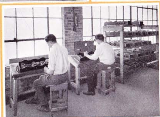
First inspection and electrical test.
