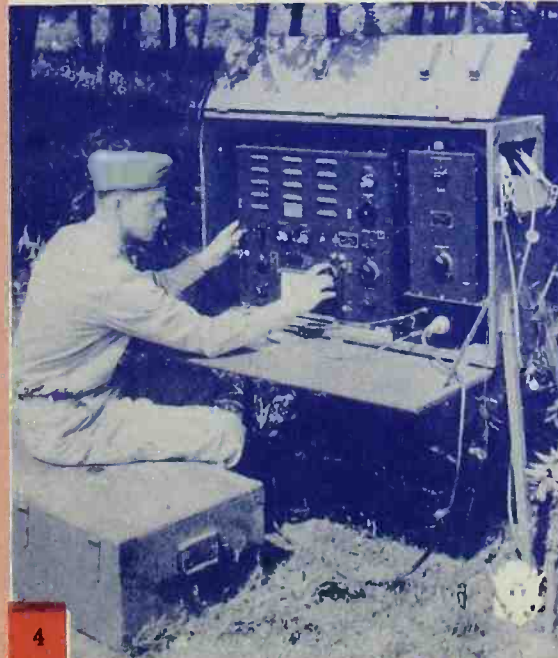
4 Close-up of Army Field transmitter.
