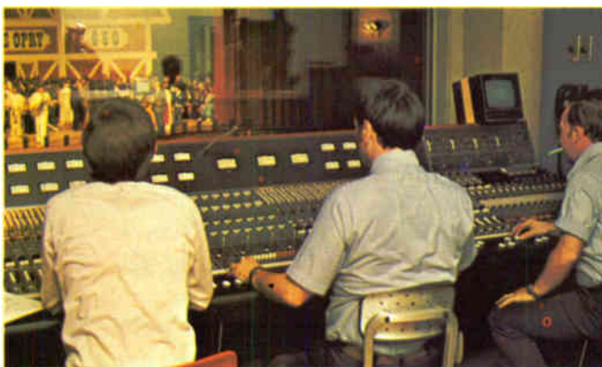
This multi-channel broadcast-recording console keeps the Opry beaming to millions of listeners.
