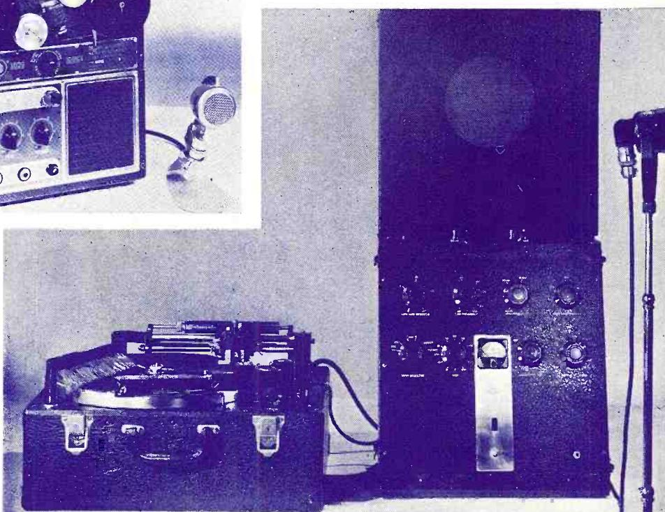
The conventional type disc recorder (left) with amplifier.
