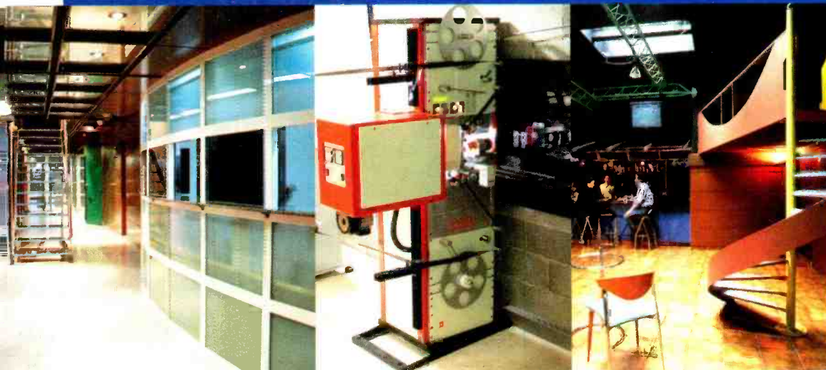
Above: the AMS Neve DFC in Soundtrack's flagship room. Below centre: the 'continuous' projector will hold 14,000ft of film
