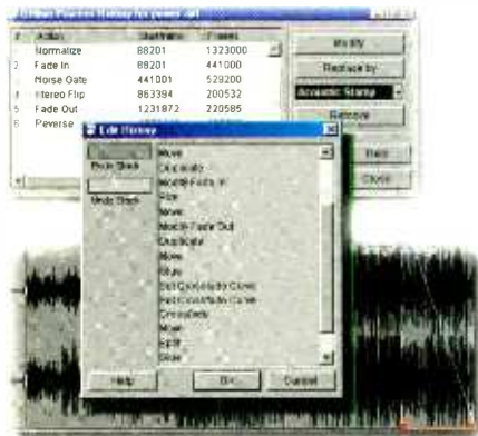
"The top grayed section of the Edit History window indicates events you can Undo or Redo, while the Offline History window behind it shows the various processes that can be modified, replaced or removed for each audio segment."
