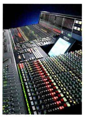
other consoles. Snapshots are recalled absolutely instantly, with no 'rippling' across the console. The immediacy of operation is the most important benefit to broadcast users. The new faders come with the useful 4-character display to show grouping and a slightly different feature set, such as backstop stereo PFL. The redesigned display is far less complicated than the sister consoles' displays, as befits the broadcast situation.
