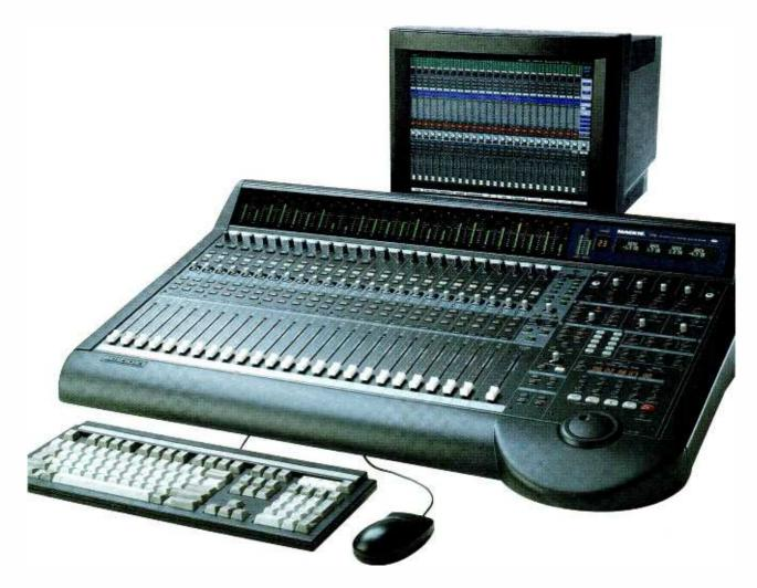
10 stereo sources can be on 10 consecutive single fader strips. Reassignment is simply achieved by clicking the fader number on screen. A window offers the choice of all possible assignments and you just click on the one required. The original number is also displayed to help return things to normal if you get lost. The meters do not follow this reassignment since they are tied to physical inputs.
