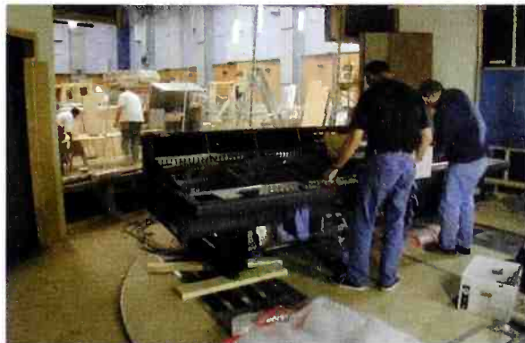
9. Reinstalling the Neve VRP Legend with VSX film panels—we refurbished it and expanded it from 64 channels to 72, to fill the frame. (Week 16)
