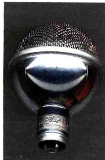
Acos-soc showing the 'reslo' type connector used on the MC2
