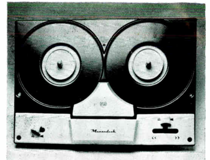
The deck, with its two controls, is as neat and as simple as it looks here with cover plate in position.
