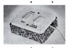
The Simon SP/4 Remote Control Unit is now available. This useful Accessory controls the Recorder in Start, Stop and Track-change functions and may be used either during record or replay. Size 1½ × 2½ × 3½ in. Price £3 3s. with cable.
