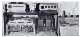
The enthusiast whose equipment is shown here is able to record from radio or disc. Stereo record/playback is also possible using the stereo tape machine on the right, and the record player (not shown).
